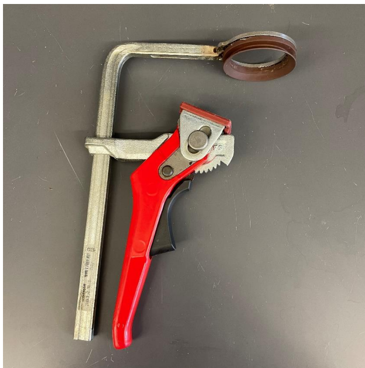
Figure 5: Bar-clamp sampler use for holding cobble and pressing a fixed-area circle into the top of the cobble where the algae would be scraped from.
