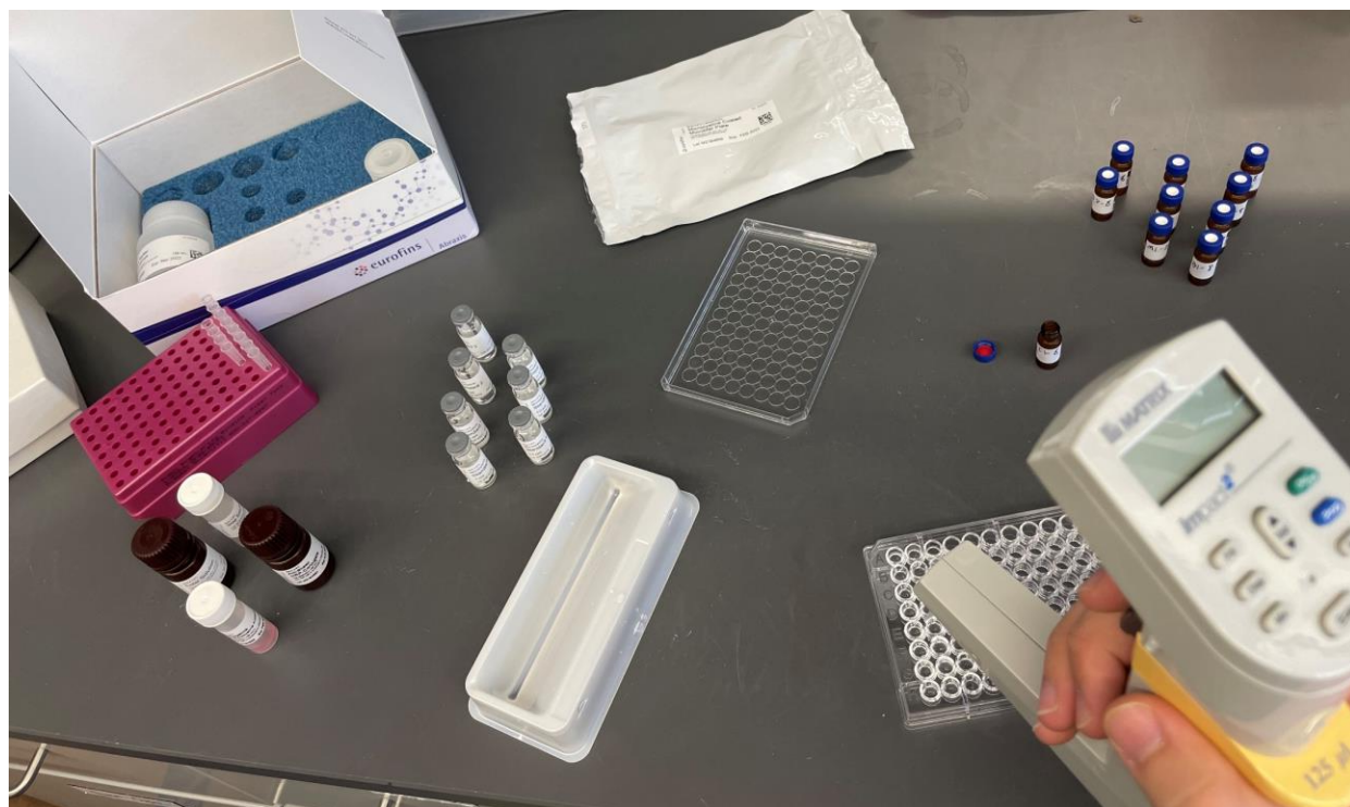
Figure 6: In process image of ELISA processing using Abraxis kits for Microcystin analysis in samples.
