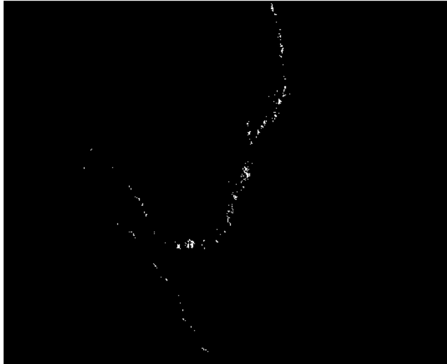
Figure 3.4: Resulting cropped binary image fire pixels of Figure 3.1 using proposed fire detection algorithm.
