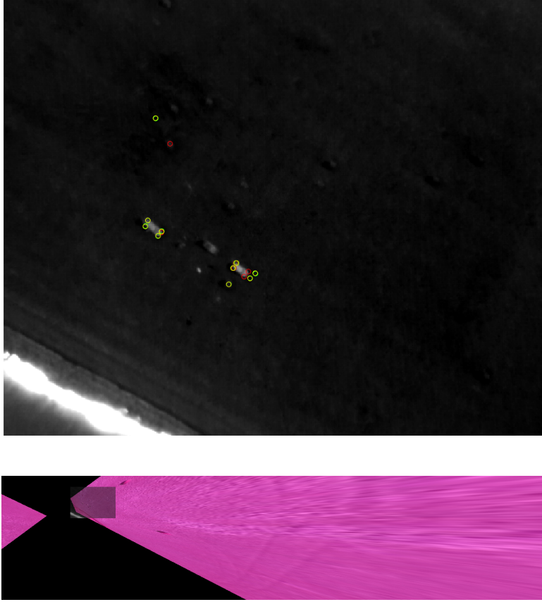
Figure 2.12: Tightly packed identified features (yellow) with respective reprojections (red) on the thermal image (top) with the estimated homography overlay (bottom).
