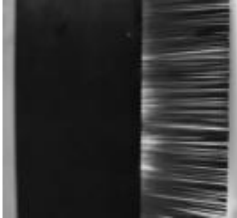
Fig. 2.13: Trailing-edge brush attached to flat plate [11]
