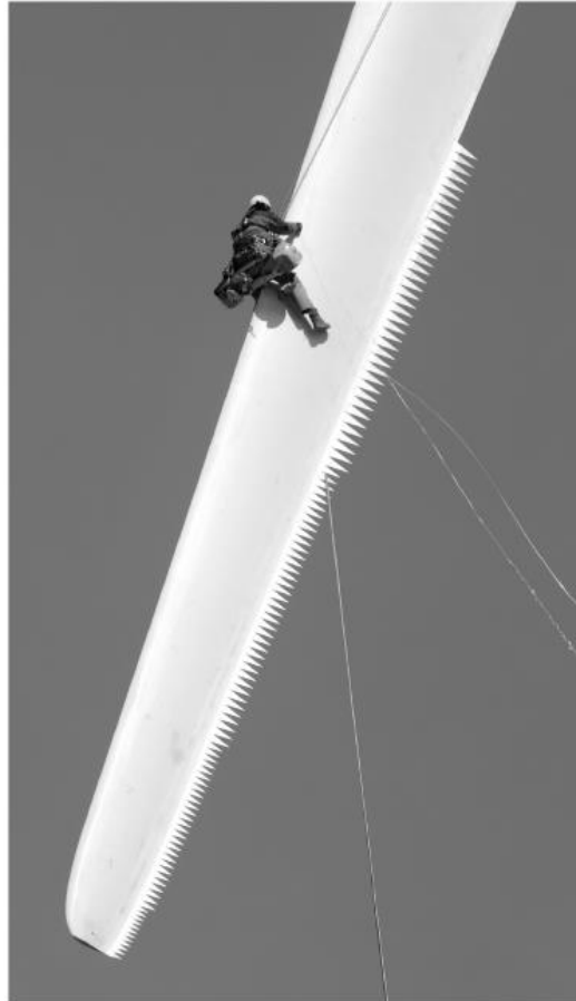
Fig. 2.5: Wind turbine blade with serrated trailing-edge [2]
