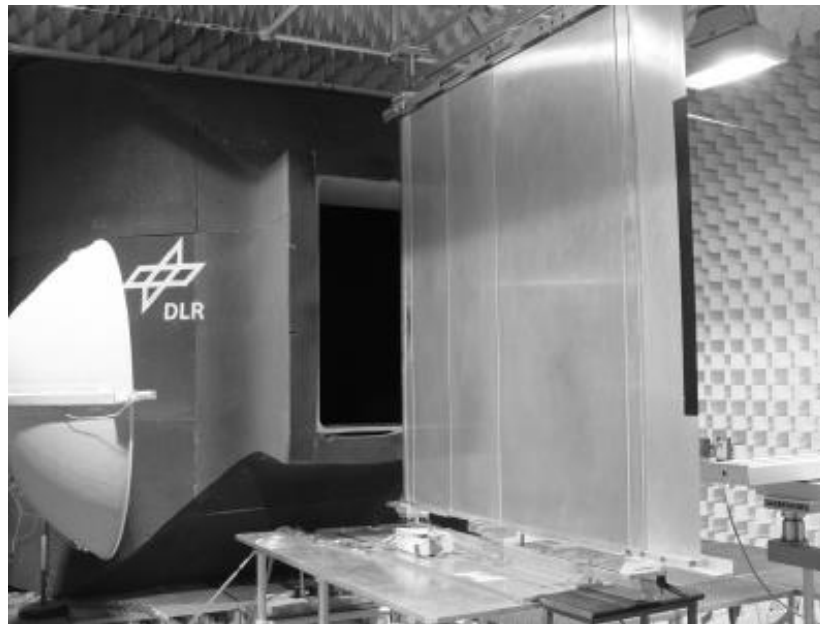
Fig. 2.12: Flat plate model in test section of DLR's aeroacoustic wind tunnel, Braunschweig [11]
