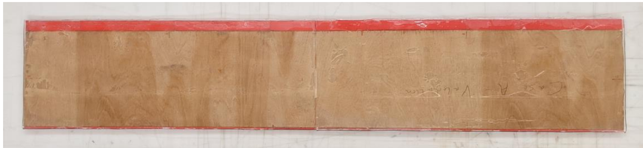
Fig. 9.32: Finished model – compliant coating applied to flat plate
