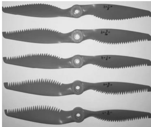
Fig. 6.1: Serrated trailing-edge propellers with varying teeth depths [70]
