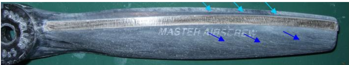
Fig. 6.5: Boundary layer trip at 10% chord of UAV propeller. [73]
