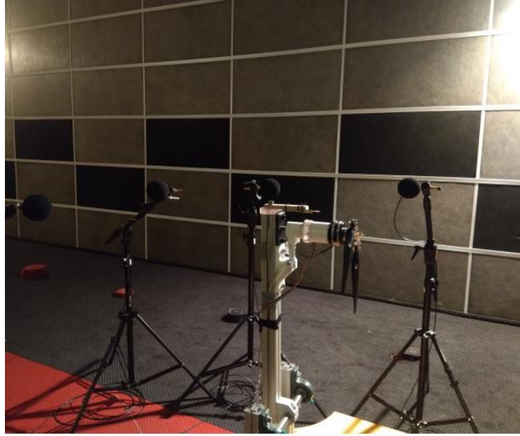
Fig. 6.12: Noise measurements from a variable pitch propeller in the anechoic test chamber at the Institute of Turbomachinery, Poland [79]
