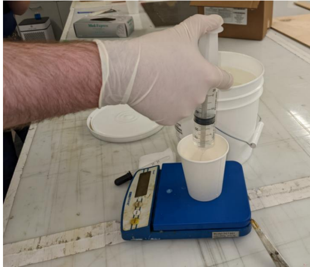
Fig. 9.2: 180 grams of base materials transferred to a cup
