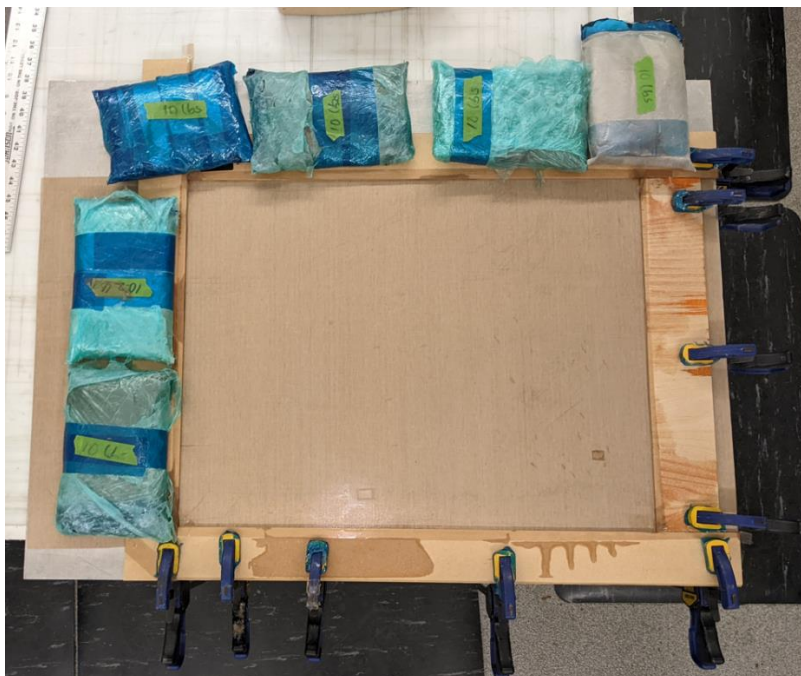
Fig. 9.12: Sand bags and clamps to keep mold intact
