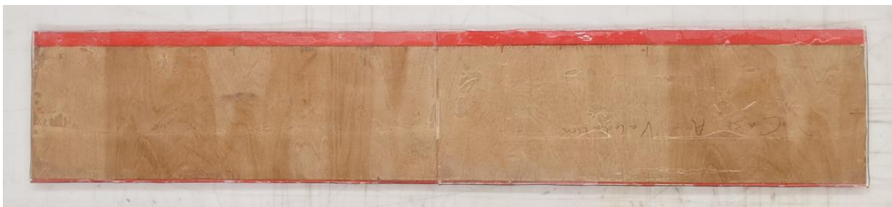
Fig. 6.20: Compliant coating applied on flat plate surface
