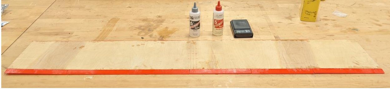
Fig. 9.25: Leading-edge and trailing-edge attached to flat plate geometry
