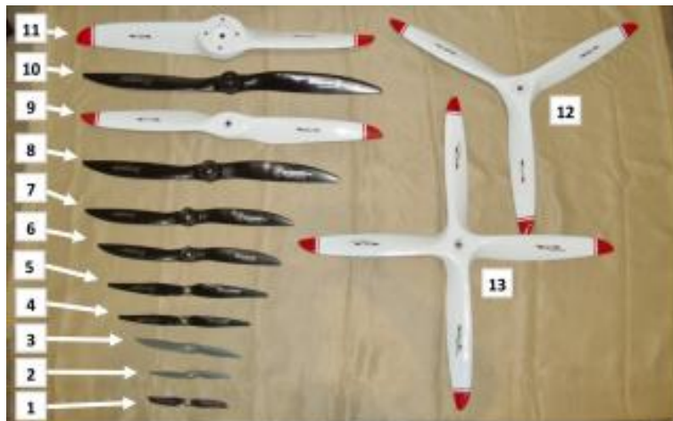
Fig. 6.4: Propellers of different diameters tested for noise measurements [72]
