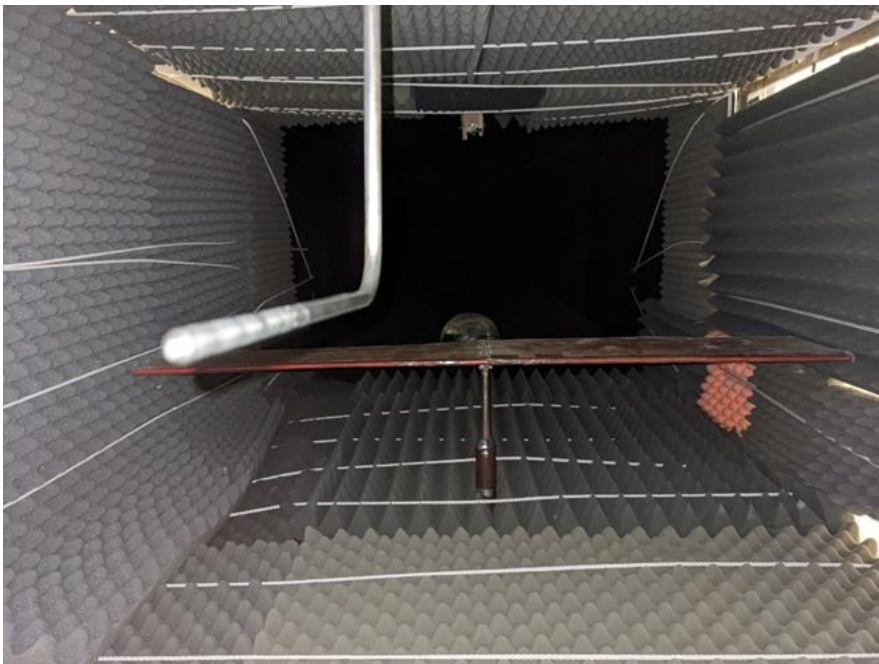
Fig. 6.31: Flat plate with compliant coating inside wind tunnel test section
