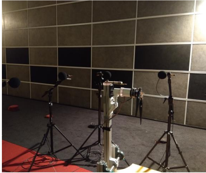
Fig. 7.2: Noise measurements from a KDE propeller in the anechoic test chamber at the Institute of Turbomachinery, Poland [79]
