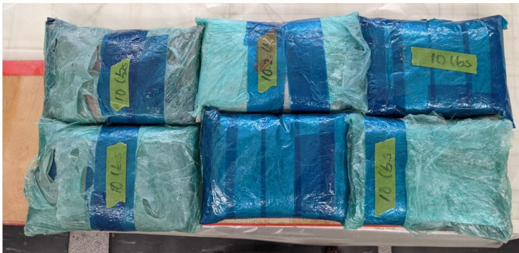
Fig. 9.30: Sand bags used to apply pressure on compliant coating
