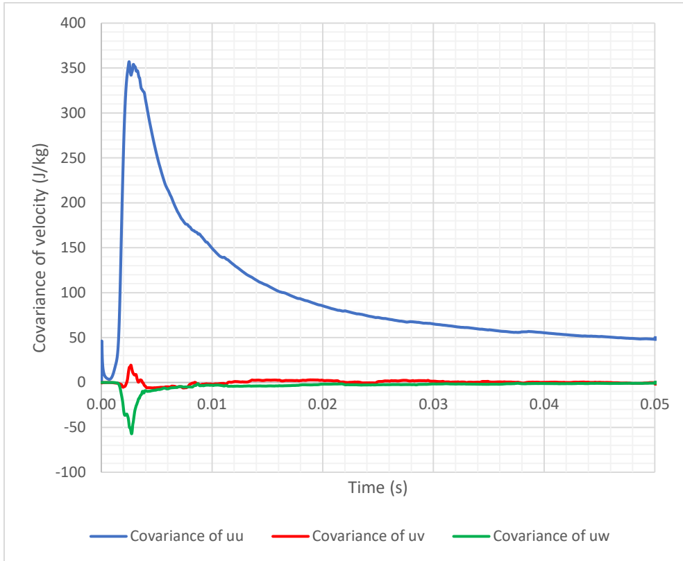
Fig. 4.29: Co-variance of velocity 10 mm downstream of trailing-edge
