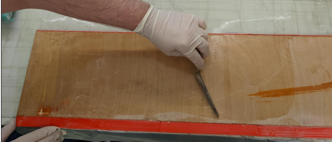
Fig. 9.27: Binding mixture applied on left side of flat-plate surface
