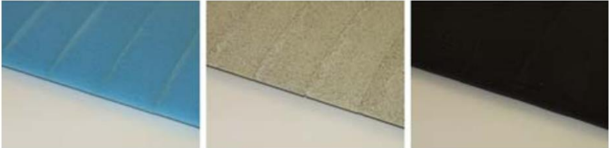
Fig. 2.14: Different porous airfoils used in the experiment [12]
