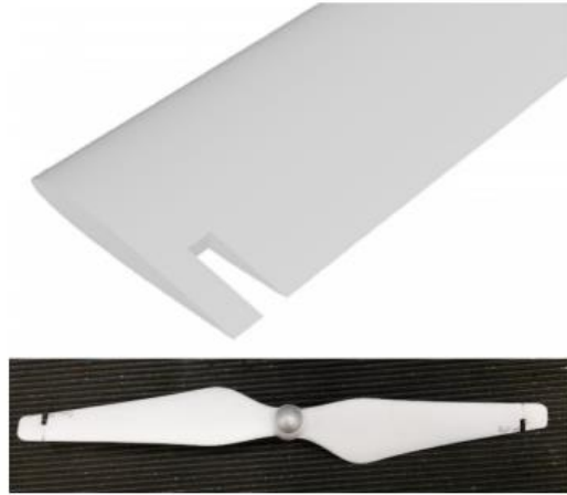
Fig. 6.3: Trailing-edge notches used for propellers of Phantom 2 quadcopter [71]
