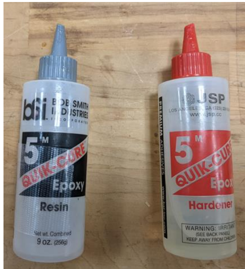
Fig. 9.22: Five-minute epoxy resin and hardener
