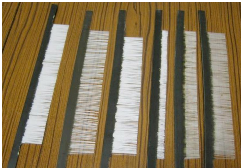
Fig. 2.11: Trailing-edge brushes with single row of polypropylene fibers [10]
