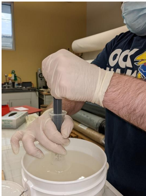
Fig. 9.1: Using syringe to transfer base material
