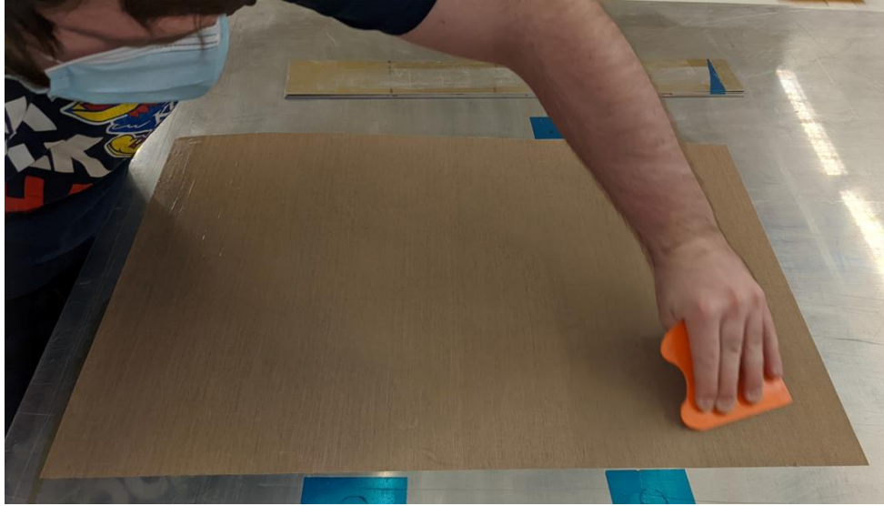
Fig. 9.10: Remove any air-pockets formed while laying the tape
