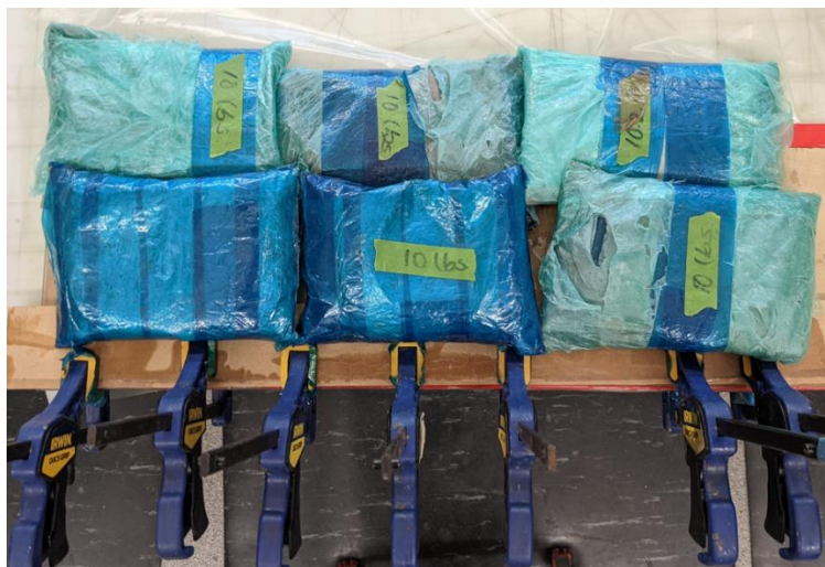
Fig. 9.28: Sand bags used to apply pressure on compliant coating
