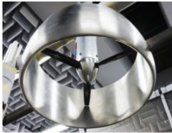
Fig. 6.10: Effects of duct around a UAV propeller investigated at TU Delft [77]
