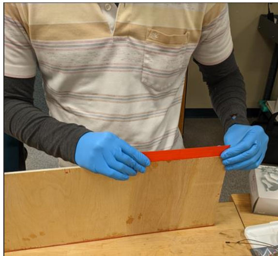
Fig. 9.24: Trailing-edge attached to flat plate using epoxy resin
