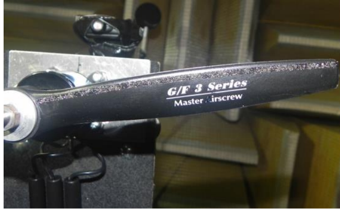
Fig. 6.11: Grit-type boundary layer trip applied near leading-edge of propeller [78]
