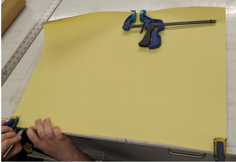
Fig. 9.8: Peel back layer of the teflon release tape
