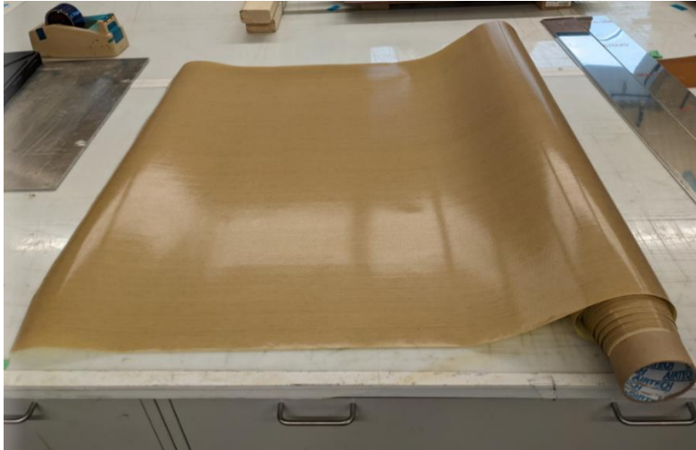
Fig. 9.6: Teflon release tape used to create base of mold
