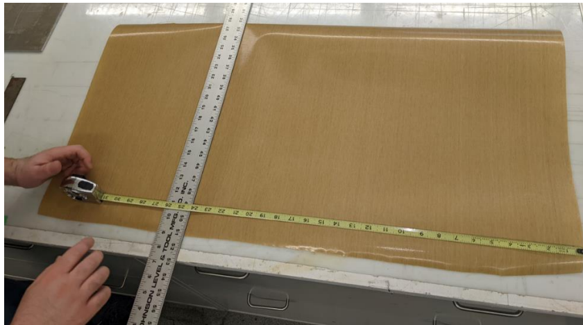
Fig. 9.7: Teflon release tape cut to dimensions of 24.1"x18.4"
