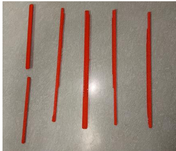
Fig. 9.20: Leading-edge pieces before sanding
