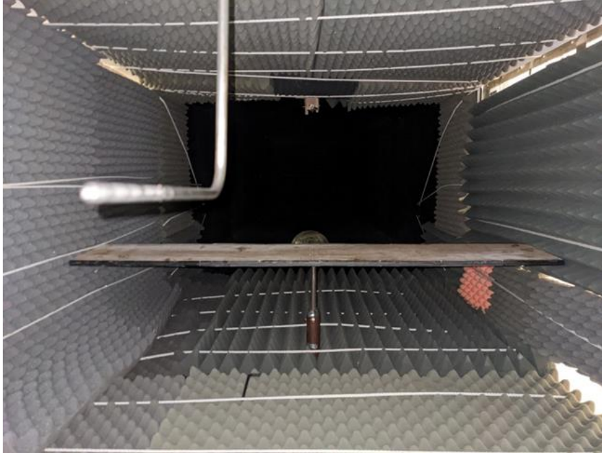
Fig. 6.30: Baseline flat plate inside wind tunnel test section
