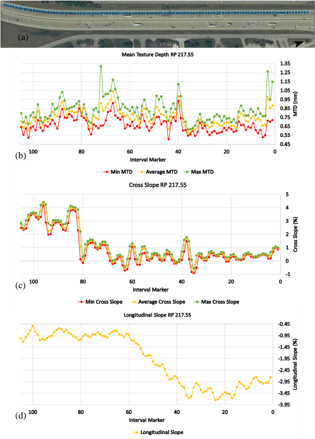
Figure 31: Scan locations (a), MTD (b), cross slope (c), and longitudinal slope (d) for RP 217.55 section.
