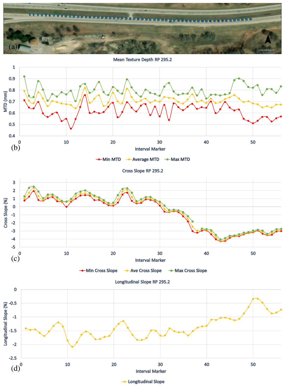
Figure 33: Scan locations (a), MTD (b), cross slope (c), and longitudinal slope (d) for RP 295.2 section.
