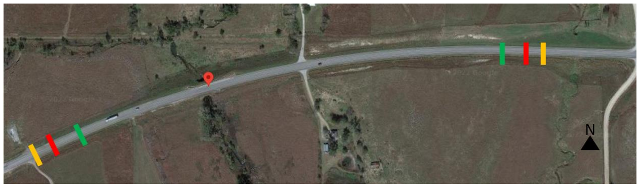
Figure 9: Approximated superelevated transitions at RP 330.1.
