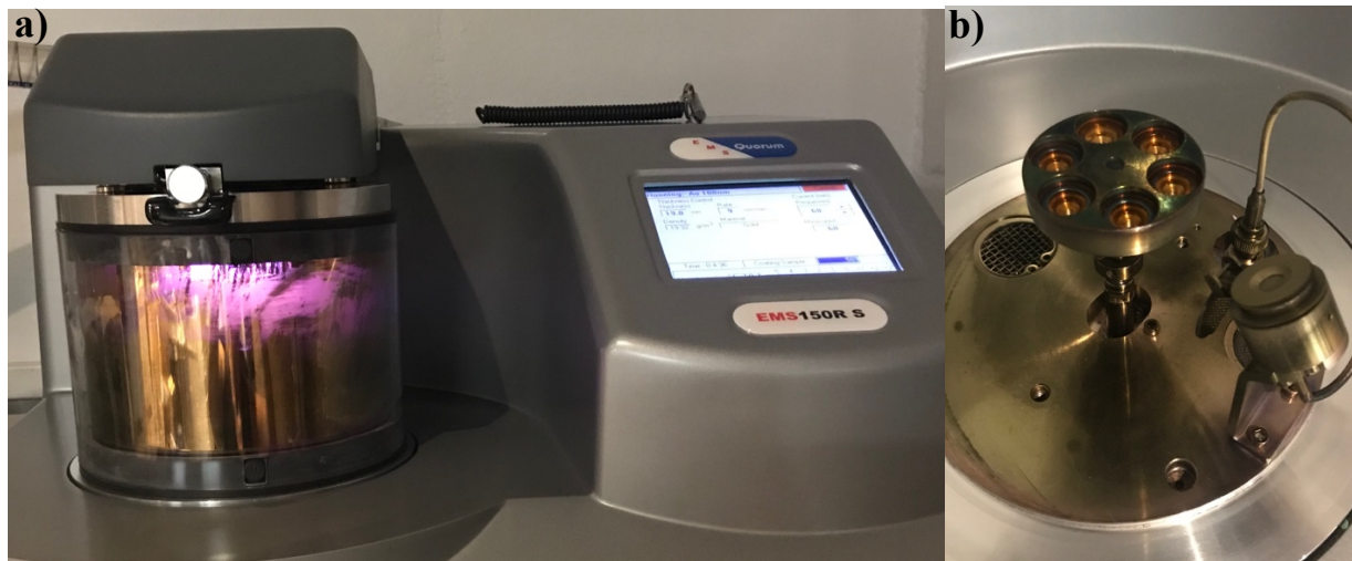
Figure 21. a) EMS150R S Quorum sputter coater used to create electrode gold layer, and b) rotational stage inside the sputter chamber.
