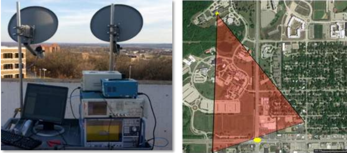
Fig. 4.4: Radar hardware instrumentation setup (left) and annotated field of view (right, courtesy of Google Maps) for measured results. The radar and intersection are depicted with a yellow star and yellow ellipse, respectively
