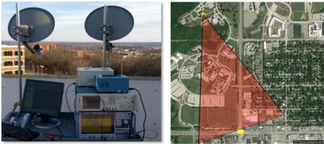
Fig. 2.30: Hardware instrumentation setup (left) and annotated field of view (right, courtesy of Google Maps) for measured results. The radar and intersection are depicted with a yellow star and yellow ellipse, respectively
