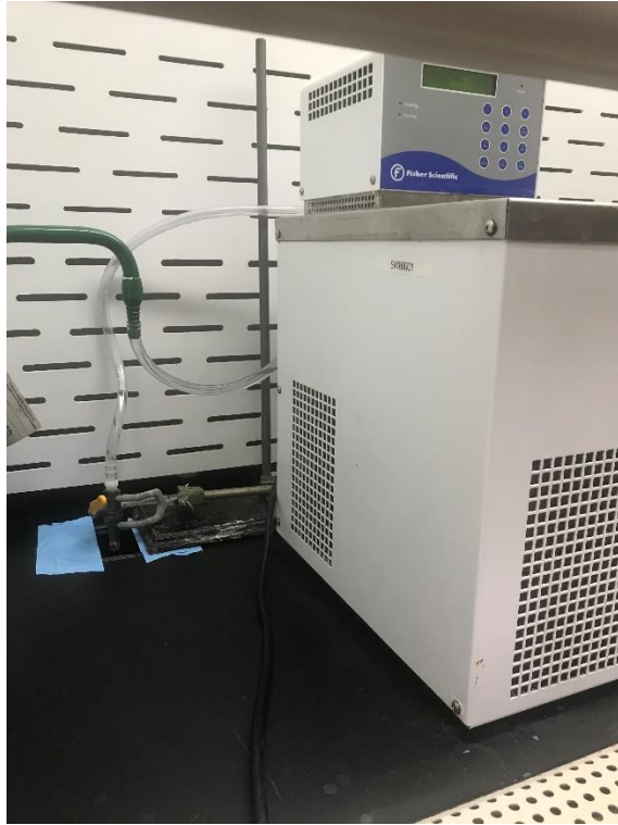
Figure 8: Test set-up for sulfuric acid tests: circulating hot water bath on left, glass dish water bath on right
