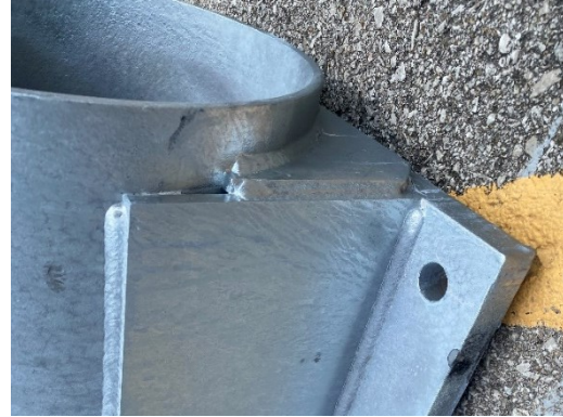
Figure 3.8. Gusseted Box Connection Welding: a) Donated Structure 165 and b) Test Specimen
