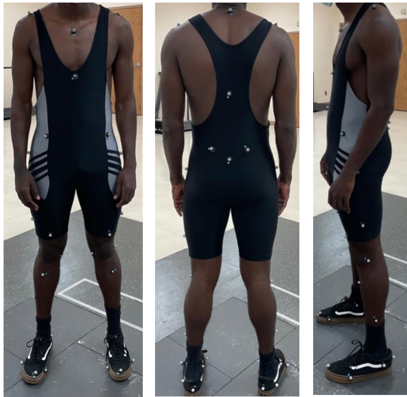
Figure 3.2: sensor placement for iWalk study. A) Frontal view. B) posterior view. C) Left lateral view
