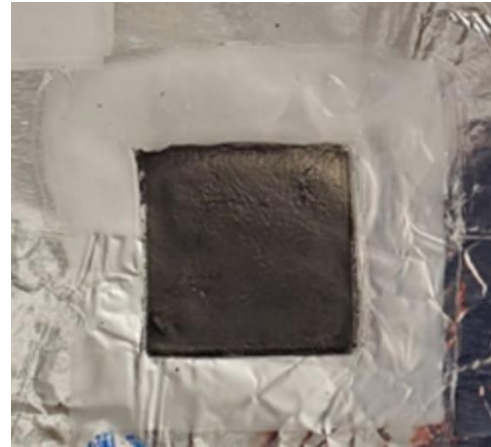
Figure 6.4: MEA fabricating via a CCM method; Post hot press procedure
