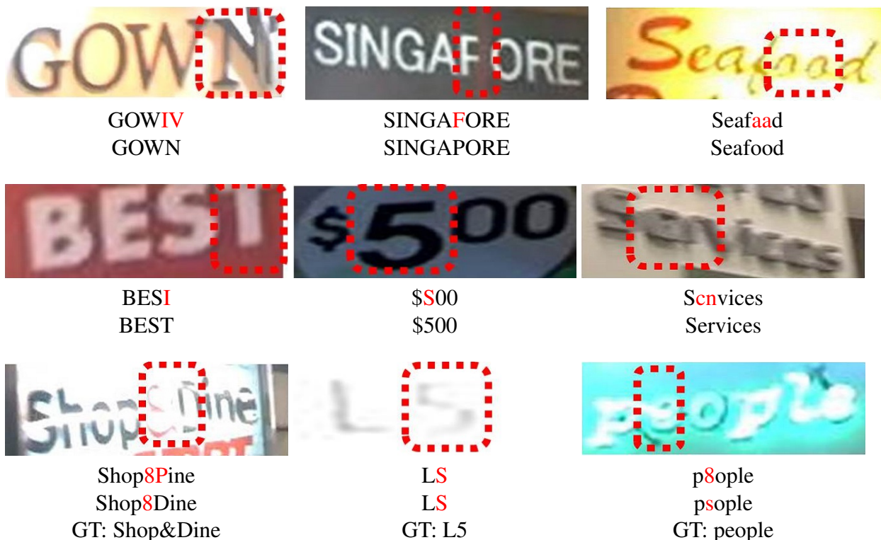
Figure 6.7: Ground truth (GT) scene-text based qualitative comparison. First two rows demonstrate the good prediction results followed by the bad recognition cases in the last row. Under each image, the first line indicates our network text prediction without using the VAB block, whereas second line shows our model with the VAB. The red-colored characters indicate the wrong predictions.
