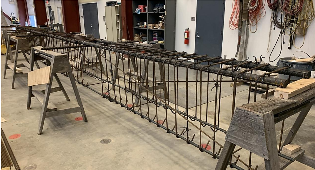
Figure 3.5: Reinforcement after assembly (18-a)
