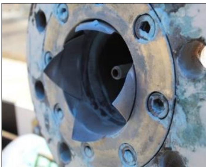
Figure 2.15. Post-test evaluation; validation that HRD rupture disc opening is complete and non-fragmenting; Test No. 1-R1 with SBC
