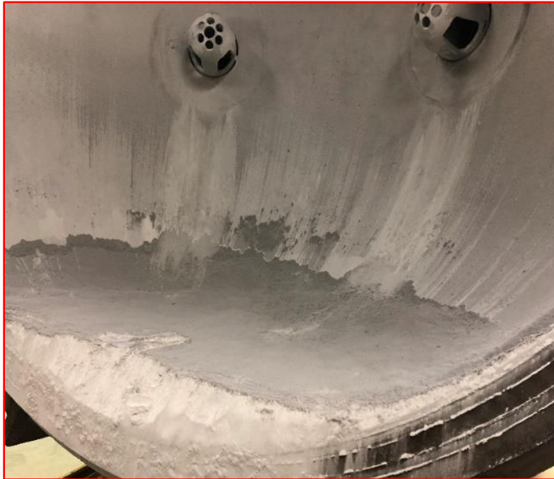
Figure 2.19. Residual combustion deposit following active suppression of aluminum powder deflagration with Met-L-X suppressant agent; Test Series 5
