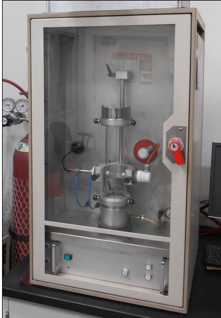
Figure 4.1. Kühner MIKE3 minimum ignition energy apparatus (photo at the permission of Fike Corporation)
