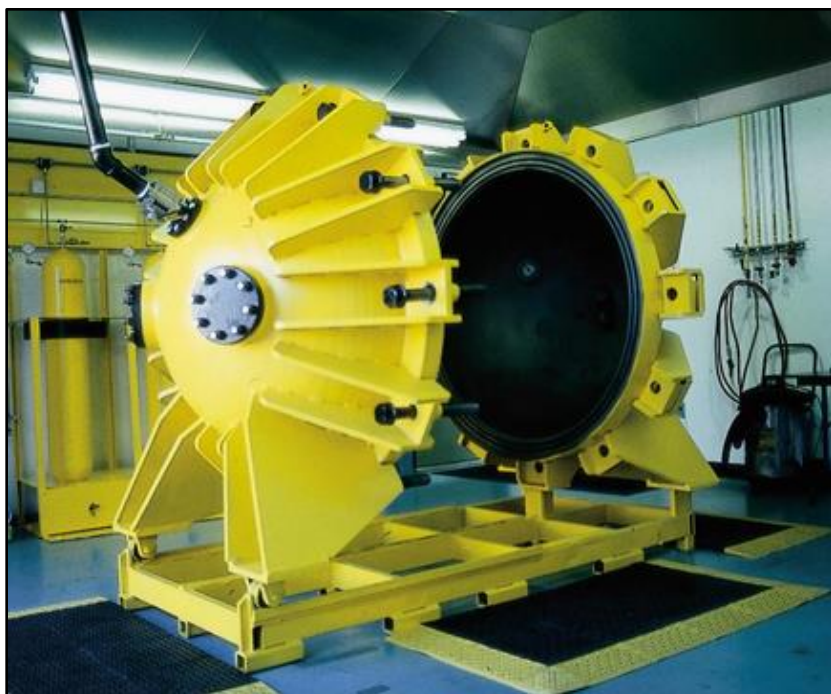
Figure 2.10. Fike Corporation 1 \text{ m}^3 combustion test vessel, utilized for fuel explosibility and active suppression testing
