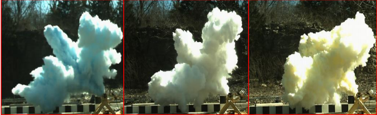
Figure 2.12. Comparison of plume geometries during open-air discharge testing, including Test No. 1-R1 with SBC (left), Test No. 2 with Met-L-X (middle), and Test No. 3 with MAP (right); images captured at 75 ms following system activation
