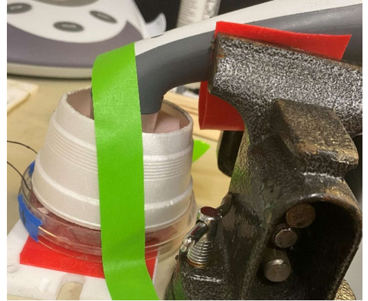
Figure 9 - Ultrasound Testing setup with probe fixed in vice and tape holding the transducer face from rising up during testing by providing slight pressure.
