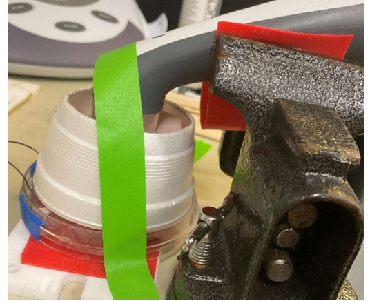
Figure 12 - Ultrasound Testing setup with probe fixed in vice and tape holding the transducer face from rising up during testing by providing slight pressure.
