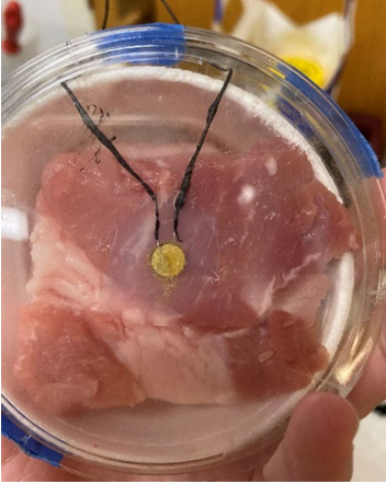
Figure 10 - Disc on petri dish with pork tissue compressed on top of coupling gel and disc to ensure a good boundary.
