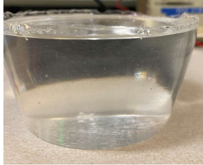
Figure 8 - Gelatin #0 from Humimic, 40 mm thick through the center
