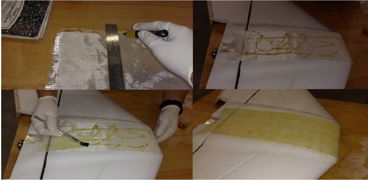
Figure 2.3: Fiberglassing the wing.
