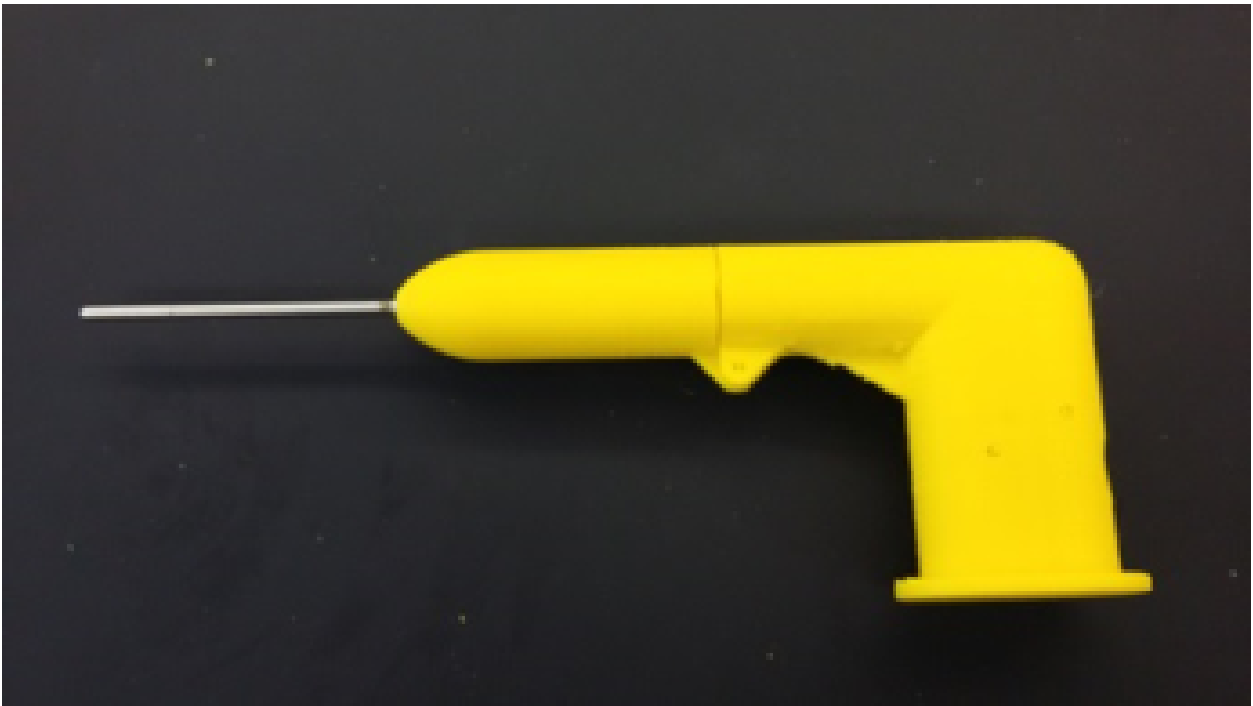
Figure 2.11: 5-hole pitot tube mount fully assembled with 5-hole pitot tube installed.
