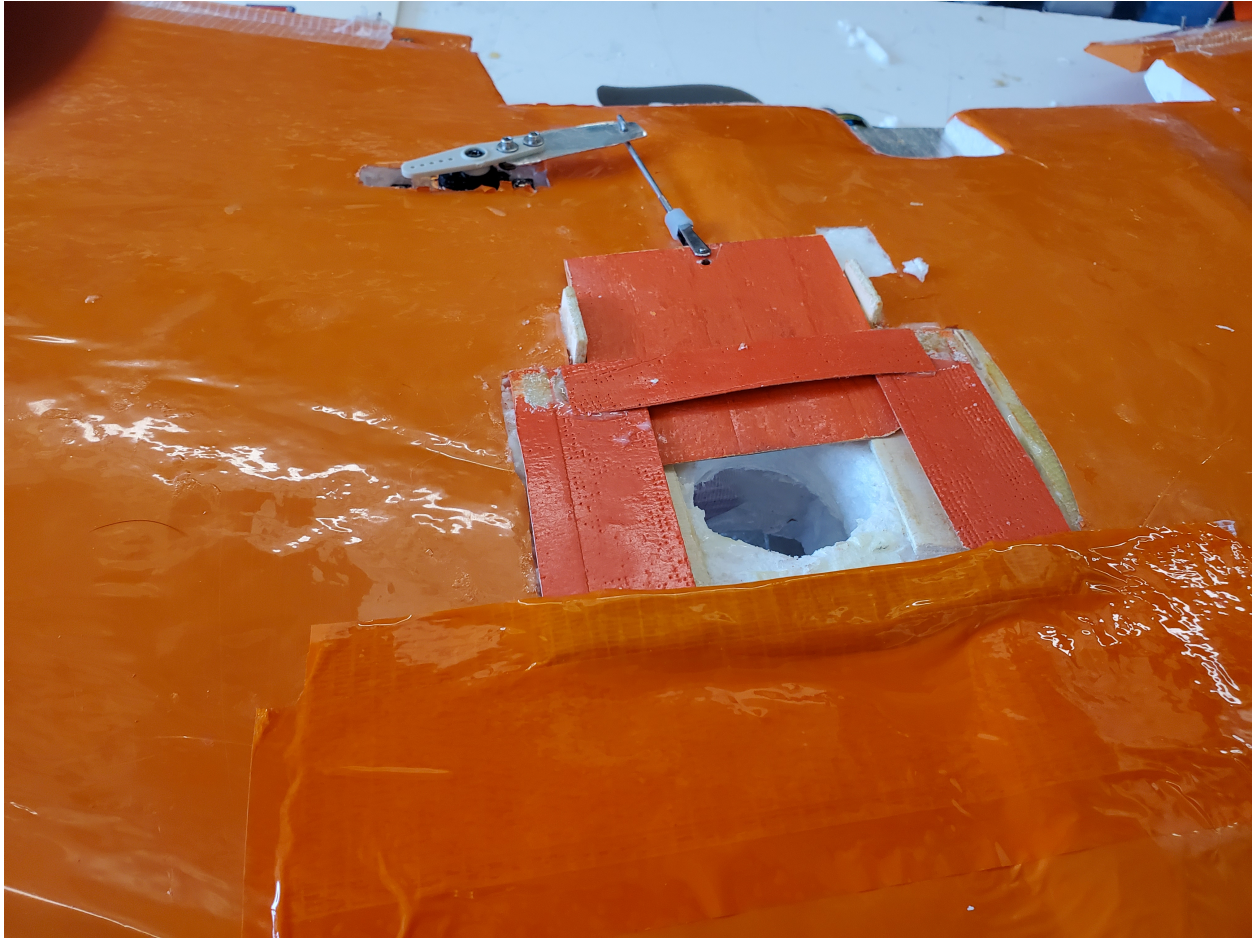
Figure 2.12: Sliding door to protect the FLir Vue Pro R thermal vision camera.
