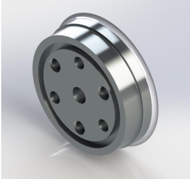
Figure 3.3.5: Ideal Bearing Mandrel Geometry
