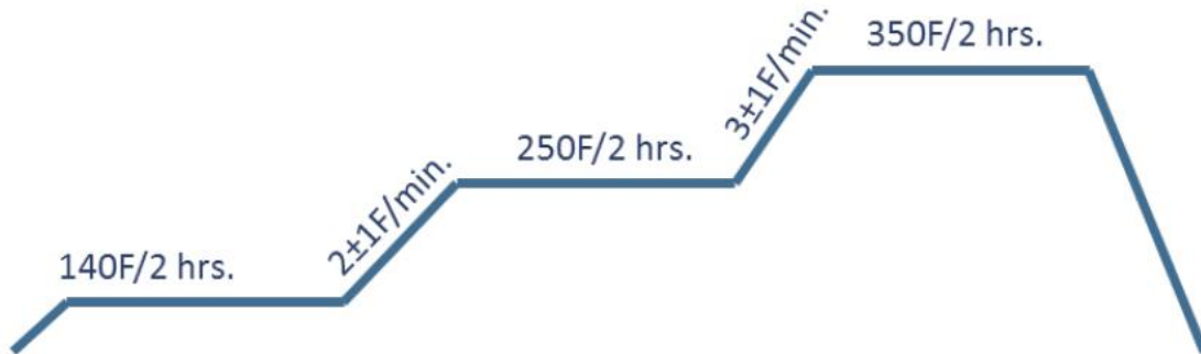
Figure 6.2.3.1: Solvay 5320-1 Cure Cycle [18]
