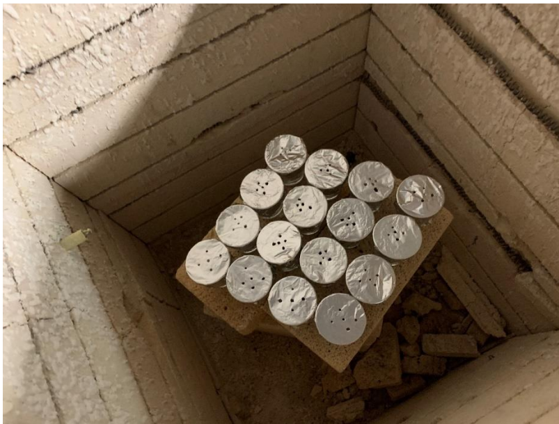
Figure 4.3.2: Test Specimen in Electric Kiln
