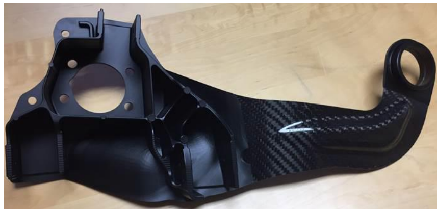
Figure 2.3.1.2: Composite Knuckle-Tie Blade [12]
