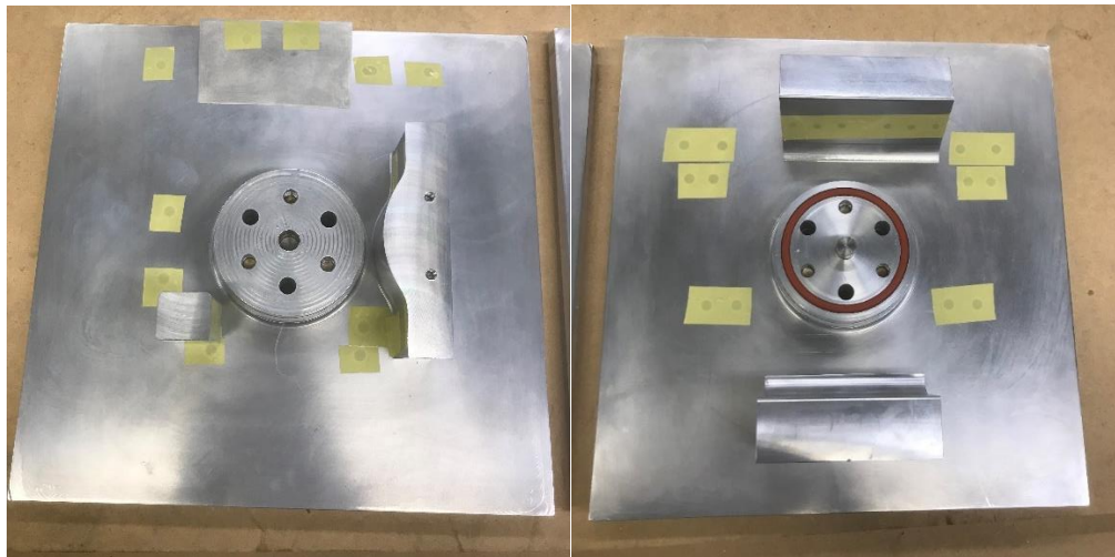
Figure 6.1.1: Tooling to Manufacture Front Left Upright
