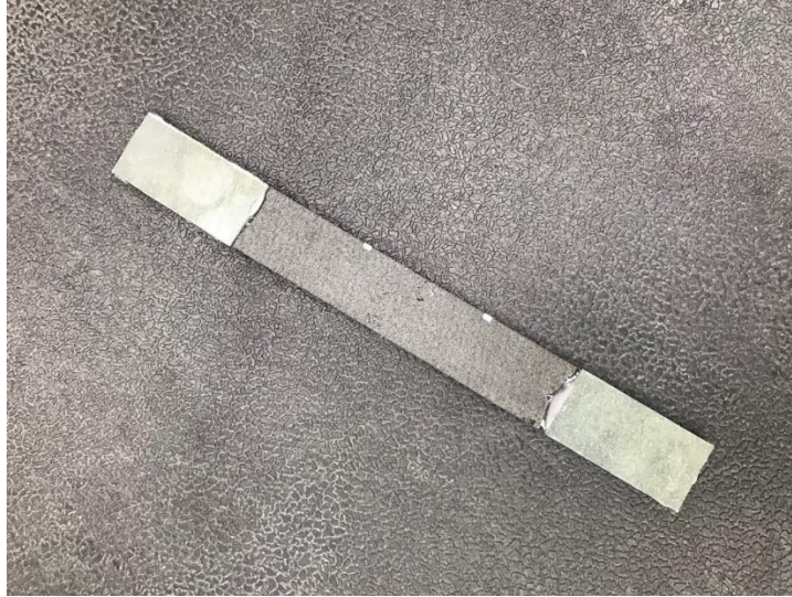
Figure 4.2.2.1: Tensile Test Coupon with Fiberglass Bonded Tabs
