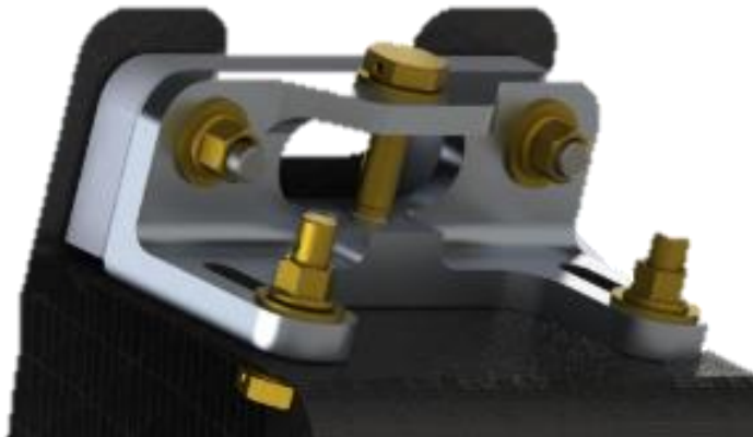
Figure 3.2.2.4: Front Upright Upper Ball Joint Mount Assembly with Shims
