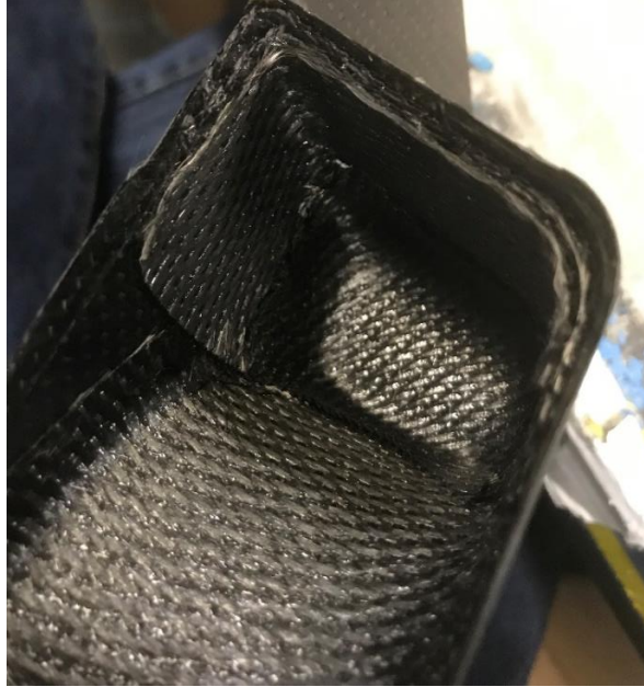
Figure 6.2.2.5: Application of Local Plies to Component
