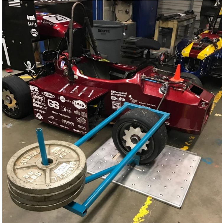
Figure 7.3.2: Maximum Lateral Load on Front Quarter Assembly
