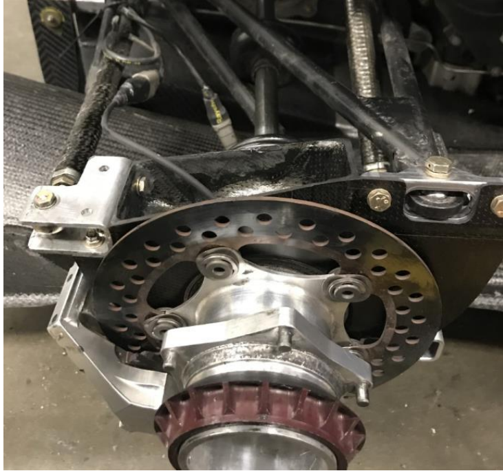
Figure 6.3.2: Fully Assembled Rear Upright
