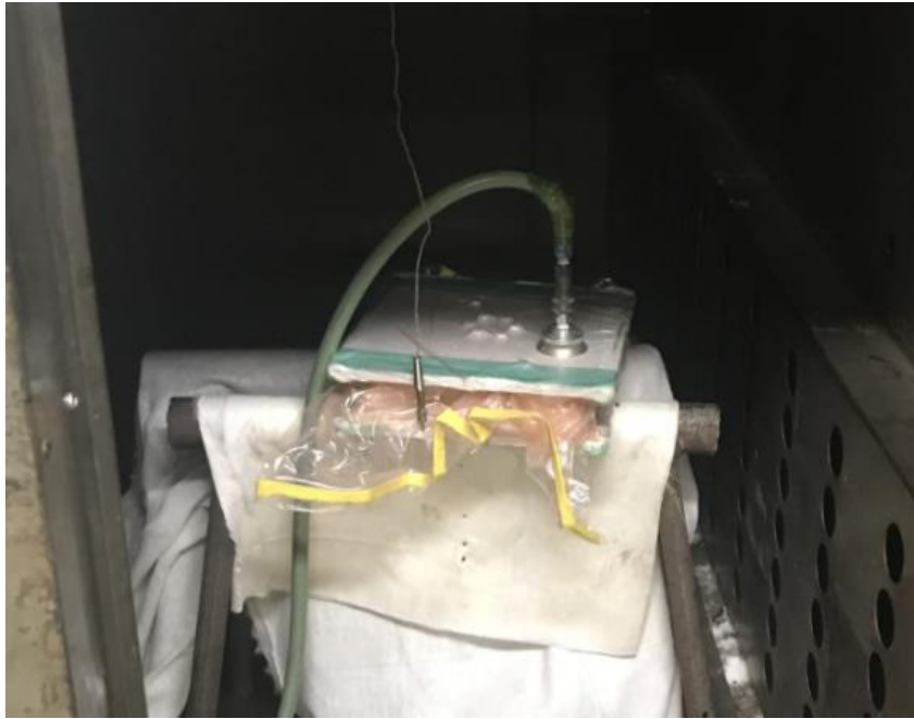
Figure 6.2.2.4: Debulking of Composite in Oven
