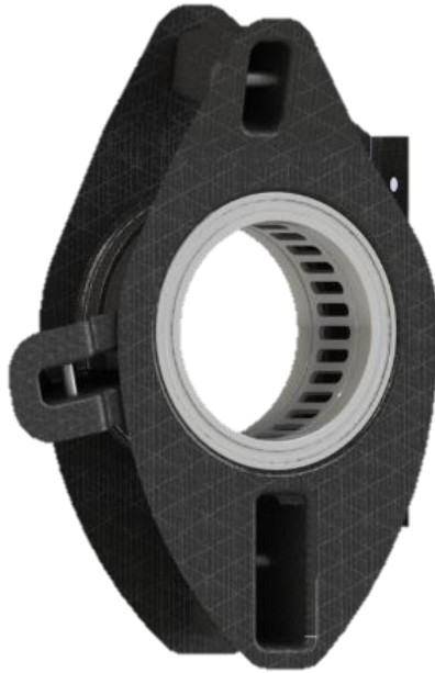
Figure 3.2.1.1: JMS Full Composite Rear Upright
