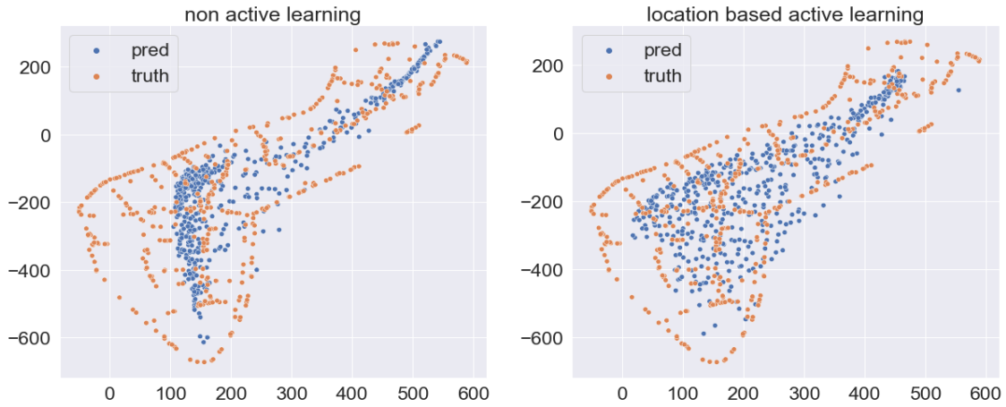
Figure 2.9: Location predictions by both the active learning and non active learning method after 25 training epochs. Compared with traditional supervised learning methods, the location based active learning makes more scattered predictions closer to the ground truths.
