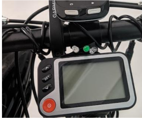
Figure 2.10 Blind spot LEDs mounted on e-bike handlebars to identify obstacles in left, center, and right lanes.
