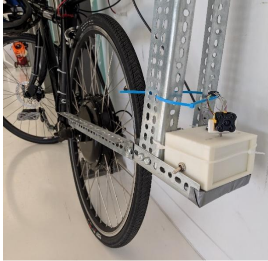
Figure 2.16 Completed 2-D lidar system mounted on the back of the electric bicycle.
