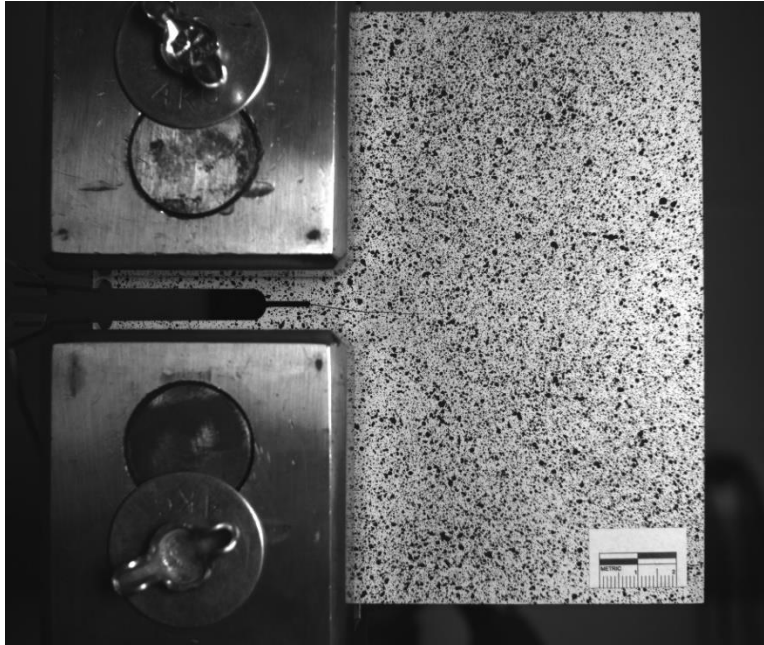
Figure A-31. C(T) specimen with 38.1 mm (1.5 in.) in-plane crack under loading case 4.
