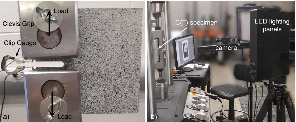
Figure 3. (a) C(T) specimen with high-contrast surface pattern; and (b) DIC hardware placement.
