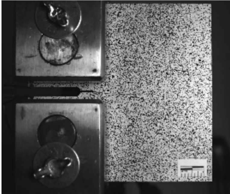
Figure A-4. C(T) specimen with 50.8 mm (2.0 in.) in-plane crack under loading case 1.
