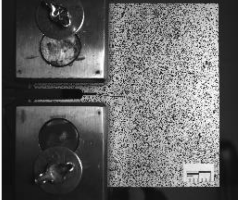
Figure A-13. C(T) specimen with 50.8 mm (2.0 in.) in-plane crack under loading case 4.
