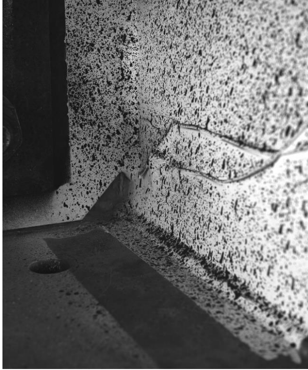
Figure 0-12. Out-of-plane specimen under loading case 3.
