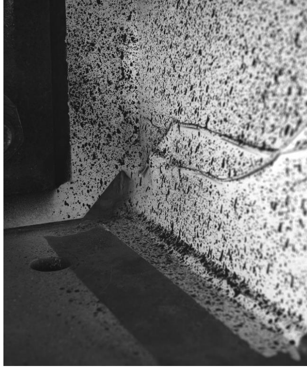
Figure 0-4. Out-of-plane specimen under loading case 1.
