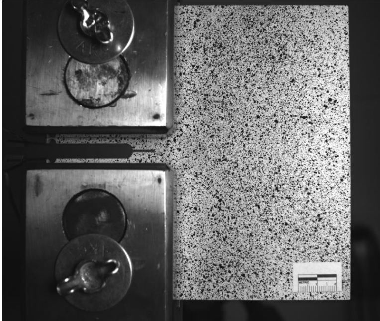
Figure A-57. Unloaded C(T) specimen with 12.7 mm (0.5 in.) in-plane crack.
