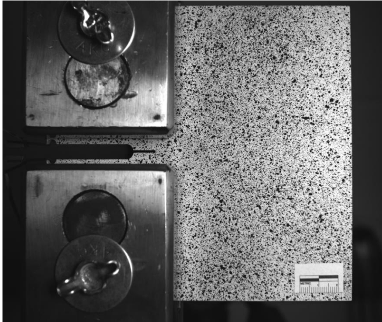
Figure A-61. C(T) specimen with 12.7 mm (0.5 in.) in-plane crack under loading case 2.
