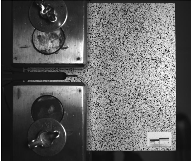
Figure A-70. C(T) specimen with 12.7 mm (0.5 in.) in-plane crack under loading case 5.
