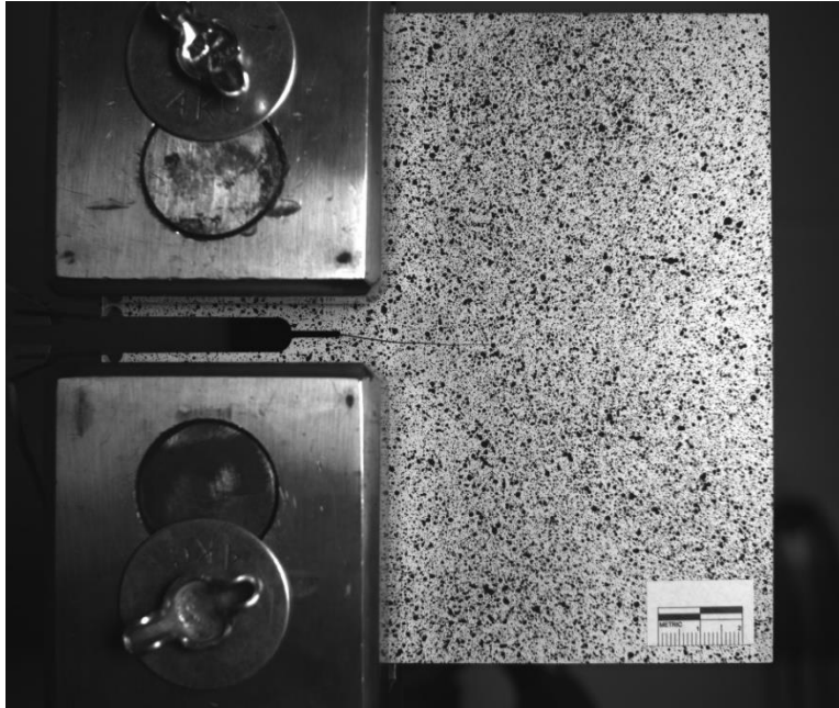
Figure A-34. C(T) specimen with 38.1 mm (1.5 in.) in-plane crack under loading case 5.
