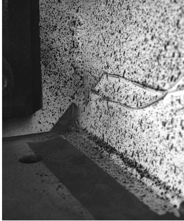
Figure 0-8. Out-of-plane specimen under loading case 2.
