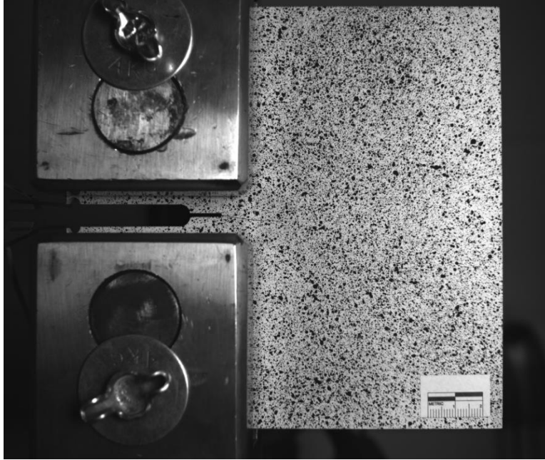
Figure A-25. C(T) specimen with 38.1 mm (1.5 in.) in-plane crack under loading case 2.
