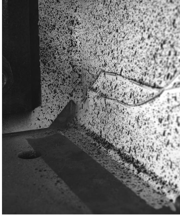
Figure 0-16. Out-of-plane specimen under loading case 4.
