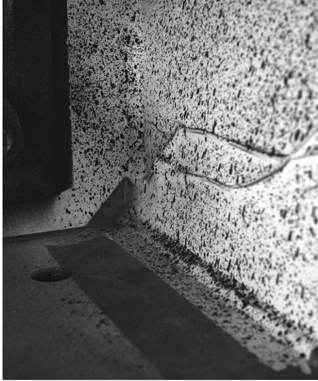
Figure 0-3. Unloaded out-of-plane specimen with 44.5 mm (1.75 in.) crack.
