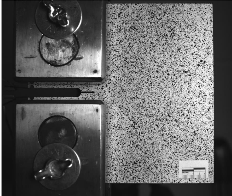
Figure A-64. C(T) specimen with 12.7 mm (0.5 in.) in-plane crack under loading case 3.
