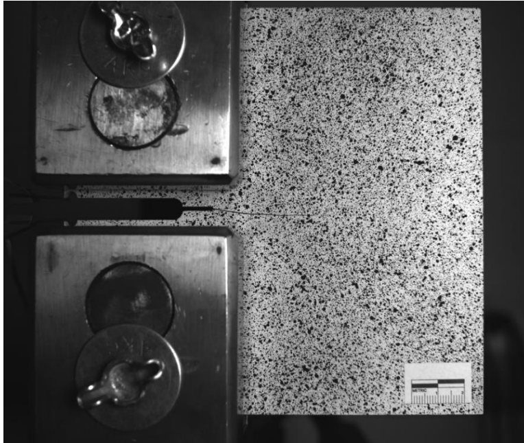
Figure A-3. Unloaded C(T) specimen with 50.8 mm (2.0 in.) in-plane crack.
