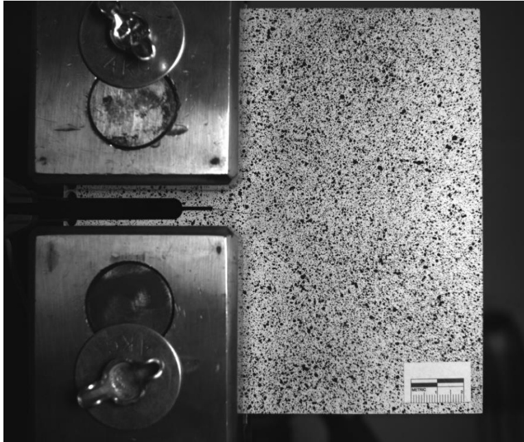
Figure A-52. C(T) specimen with 25.4 mm (1.0 in.) in-plane crack under loading case 5.
