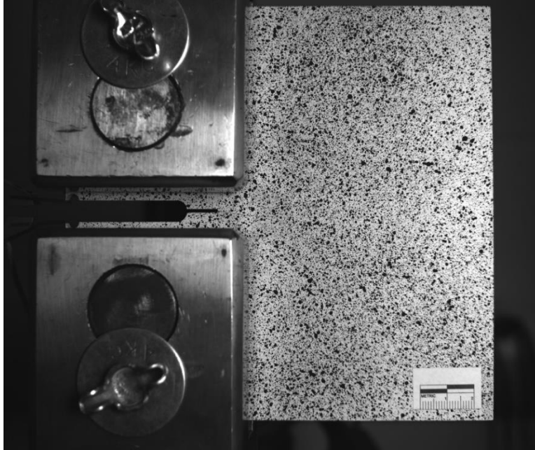
Figure A-21. Unloaded C(T) specimen with 38.1 mm (1.5 in.) in-plane crack.
