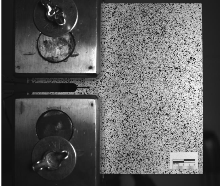
Figure A-22. C(T) specimen with 38.1 mm (1.5 in.) in-plane crack under loading case 1.
