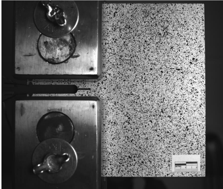
Figure A-67. C(T) specimen with 12.7 mm (0.5 in.) in-plane crack under loading case 4.
