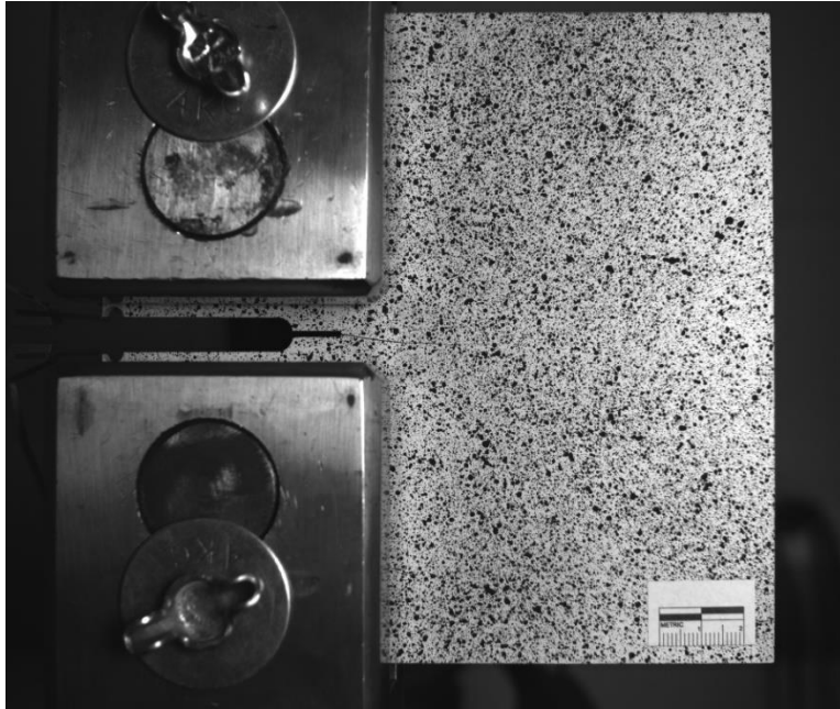
Figure A-28. C(T) specimen with 38.1 mm (1.5 in.) in-plane crack under loading case 3.
