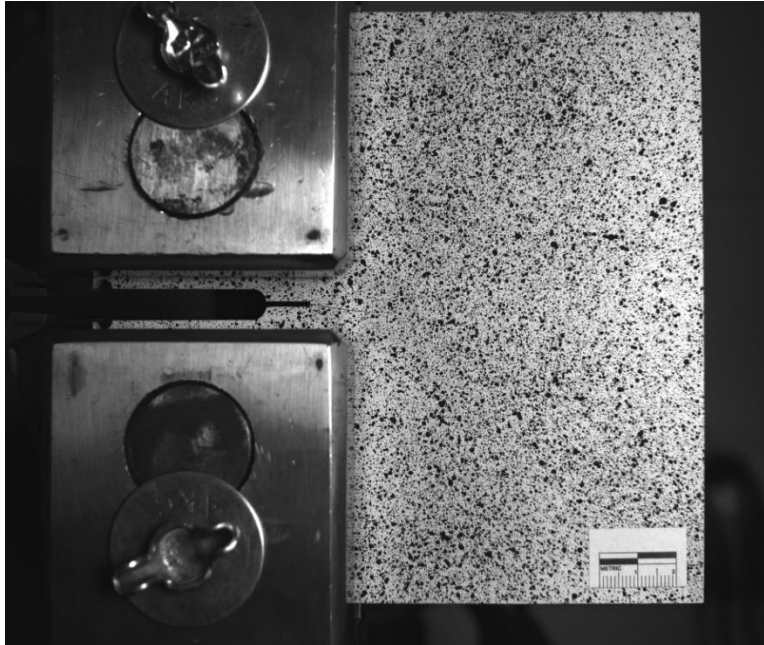
Figure A-49. C(T) specimen with 25.4 mm (1.0 in.) in-plane crack under loading case 4.
