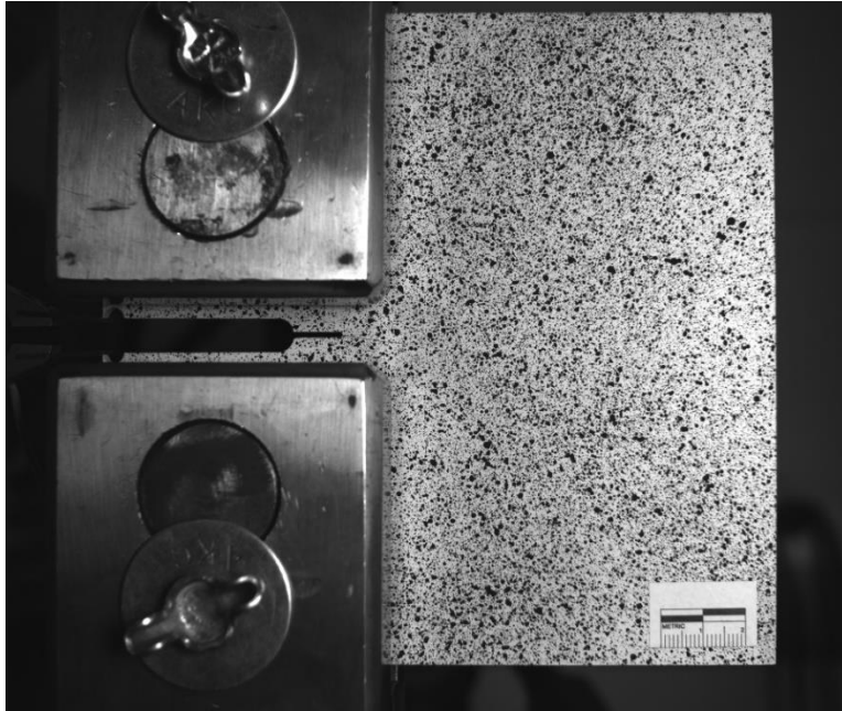
Figure A-46. C(T) specimen with 25.4 mm (1.0 in.) in-plane crack under loading case 3.
