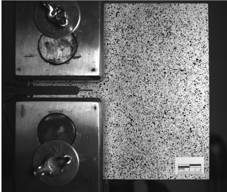
Figure A-58. C(T) specimen with 12.7 mm (0.5 in.) in-plane crack under loading case 1.
