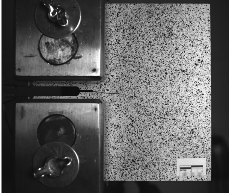
Figure A-7. C(T) specimen with 50.8 mm (2.0 in.) in-plane crack under loading case 2.
