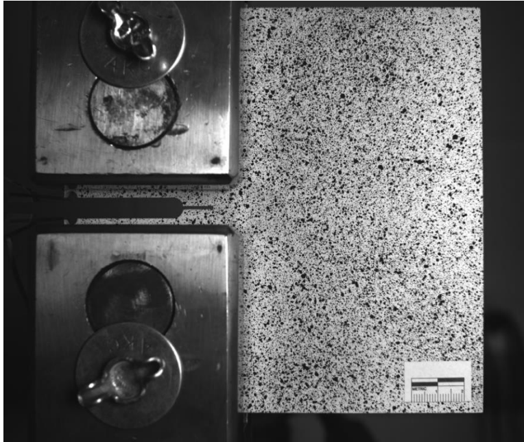
Figure A-39. Unloaded C(T) specimen with 25.4 mm (1.0 in.) in-plane crack.
