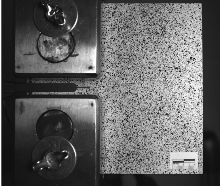
Figure A-40. C(T) specimen with 25.4 mm (1.0 in.) in-plane crack under loading case 1.
