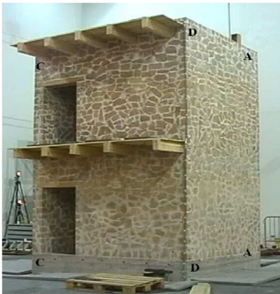
Fig. 5. Shake table test of stone masonry building in lime mortar test specimen (from Betti et al., 2015)
