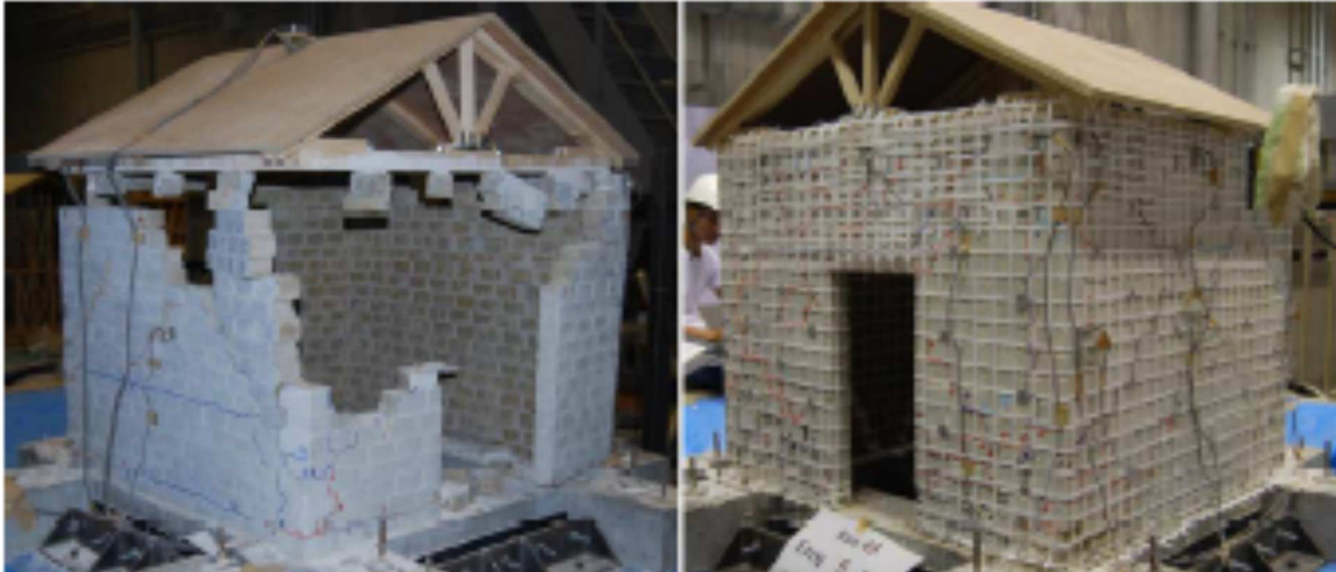
Fig. 7. Level of collapse seen in the non-retrofitted house (left) and pp-band retrofitted masonry specimens (right) (from Meguro et al., 2012).
