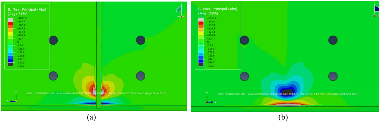
Figure 6-17: Absolute maximum principal stress [MPa] contours of the web gap region of the uncracked unretrofitted girder: (a) on the interior side; (b) on the fascia side
