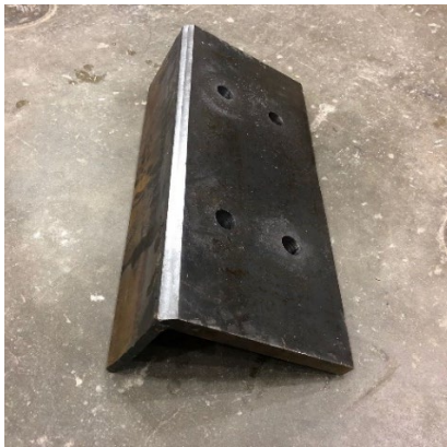
Figure 6-7 Modified steel retrofit geometry and dimensions for the combined CFRP-steel retrofit: (a) Modified angles to the south of the CP; (b) Modified backing plate
