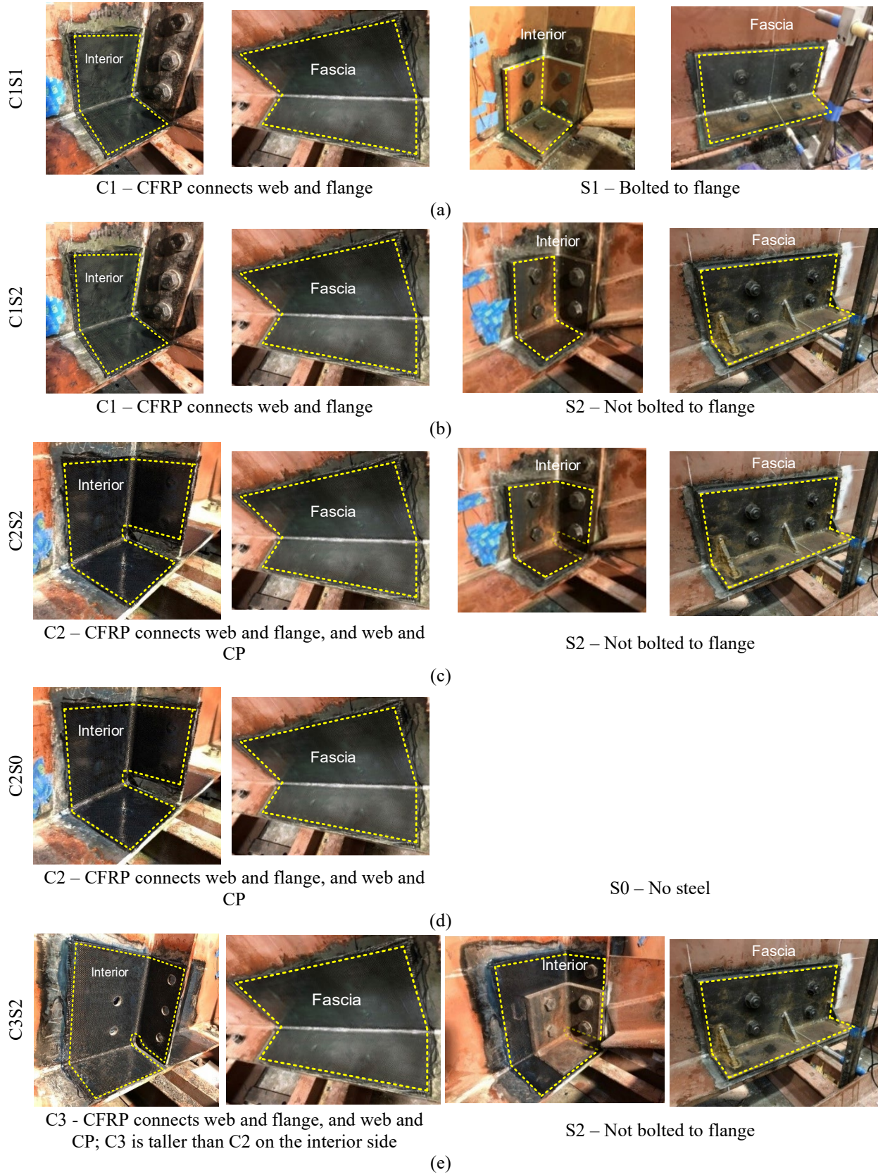
Figure 6-6 Description of repair configurations; the extents of the CFRP are shown in dashed lines
