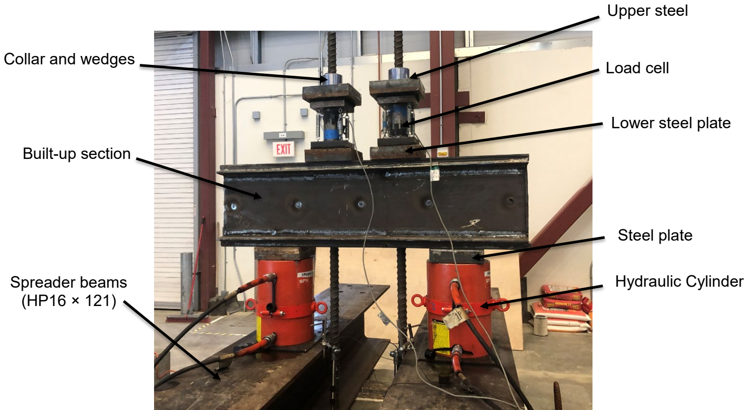
Figure 2.14 Test frame – second configuration
