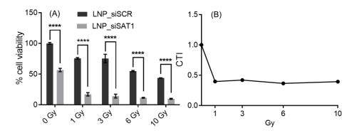
**Figure 4.** Cytotoxic response to different doses of radiation in *SAT1* KD U251 cells (**A**). The corresponding calculated CTI values (**B**) for plot a values; CTI < 0.7 indicates a significant synergistic effect. Values are expressed as the mean  $\pm$  standard error of the mean (SEM, *n* = 3). Statistical analysis was performed using two-way ANOVA, followed by Tukey's test (*n* = 3). \*\*\*\* *p* < 0.0001 (*p* < 0.05 was considered statistically significant).
