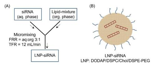
**Figure 1.** (**A**) Schematic illustration of the formulation of LNP-siRNA following micromixing in a microfluidic chamber. The flow rate ratio (FRR) of aq:org of 1:3 and a total flow rate of 12 mL/min yielded siRNA encapsulated LNP (**B**) that were in the 80 nm (PDI = 0.16) size range with neutral surface charge.
