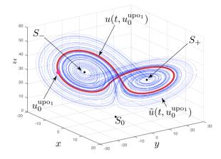
Fig. 3. Period-1 UPO  $u^{\text{upo}_1}(t)$  (red, period  $\tau_1 = 1.28701$ ) stabilized using the UDFC method, and pseudotrajectory  $\tilde{u}(t, u_0^{\text{upo}_1})$  (blue,  $t \in [0, 100]$ ) in system (2) with parameters set at r = 28, c = 10, b = 8/3.
