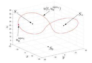
Fig. 2. Period-1 UPO  $u^{\text{upo}_1}(t)$  (red, period  $\tau_1 = 1.28701$ ) stabilized using the UDFC method in system (2) with parameters set at r = 28, c = 10, b = 8/3.
