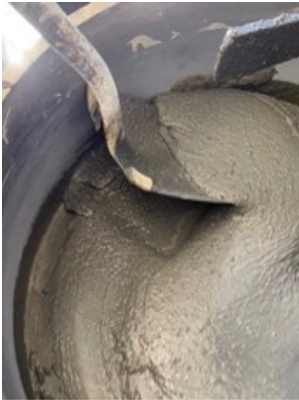
Figure 3.6: Mixture after Adding HRWR
