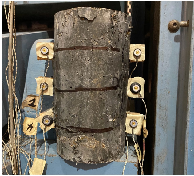
Figure 3.8: Marker Placement on Cylinder
