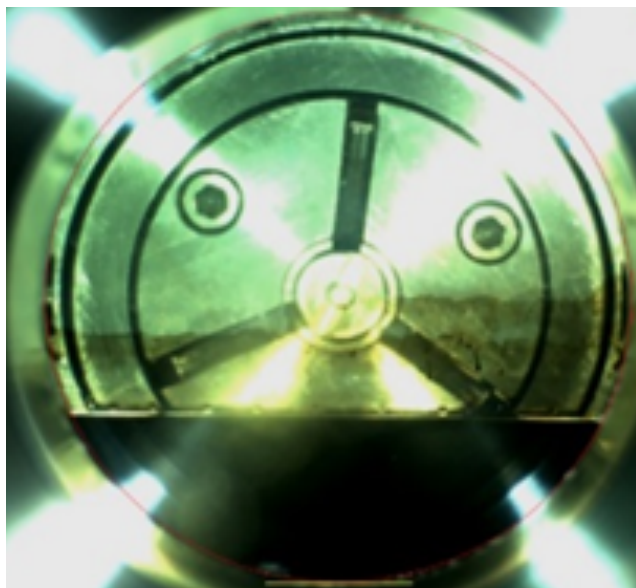
Figure 38 L 1 L 2 phase behavior at 2992.20 psi between CO 2 and oil at 120 °C
