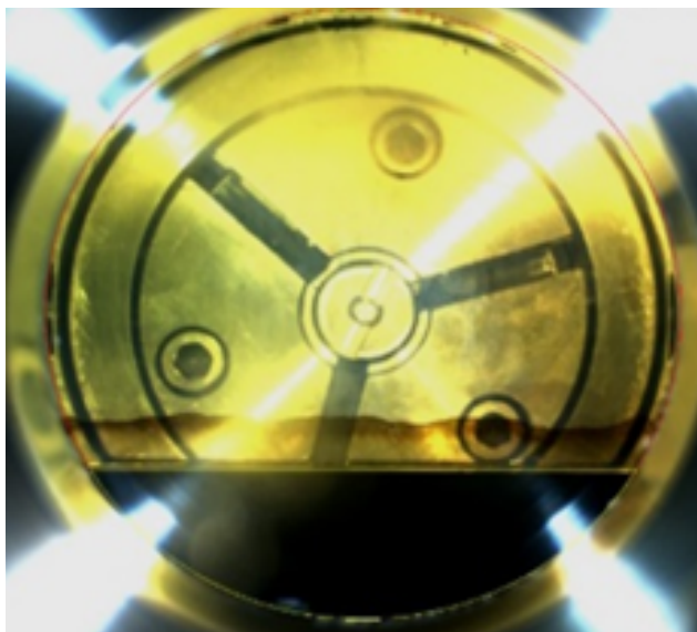
Figure 34 L_1L_2 phase behavior at 2765.64 psi between CO_2 and oil at 80 °C
