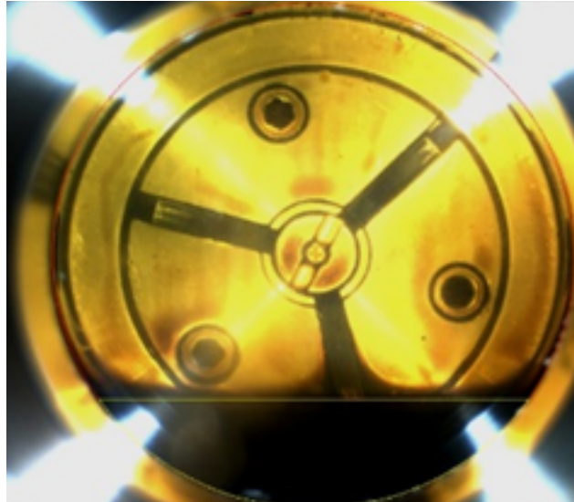
Figure 30 L 1 L 2 phase behavior at 3034 psi between CO 2 and oil at 27 °C
