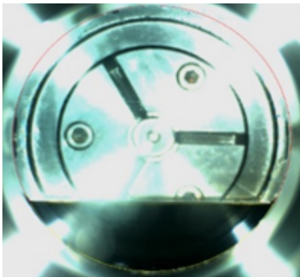
Figure 37 LV phase behavior at 2138.45 psi between CO 2 and oil at 120 °C
