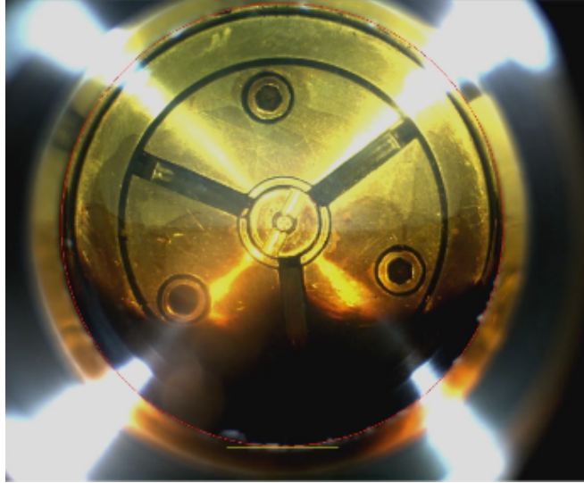
Figure 31 Oil extraction column between CO 2 and oil at 3219 psi at 27 °C
