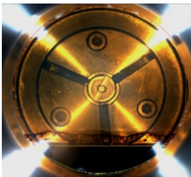
Figure 35 L_1L_2 phase behavior at 3335.52 psi between CO_2 and oil at 80 °C
