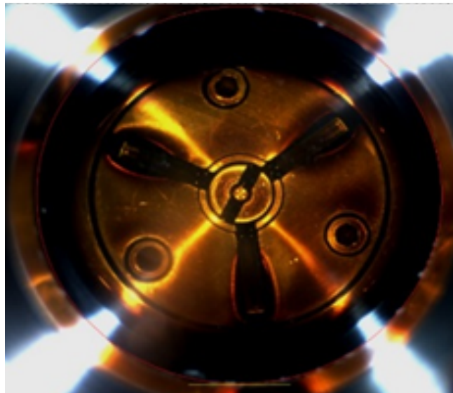
Figure 32 Miscible phase behavior at 3253 psi between CO 2 and oil at 27 °C
