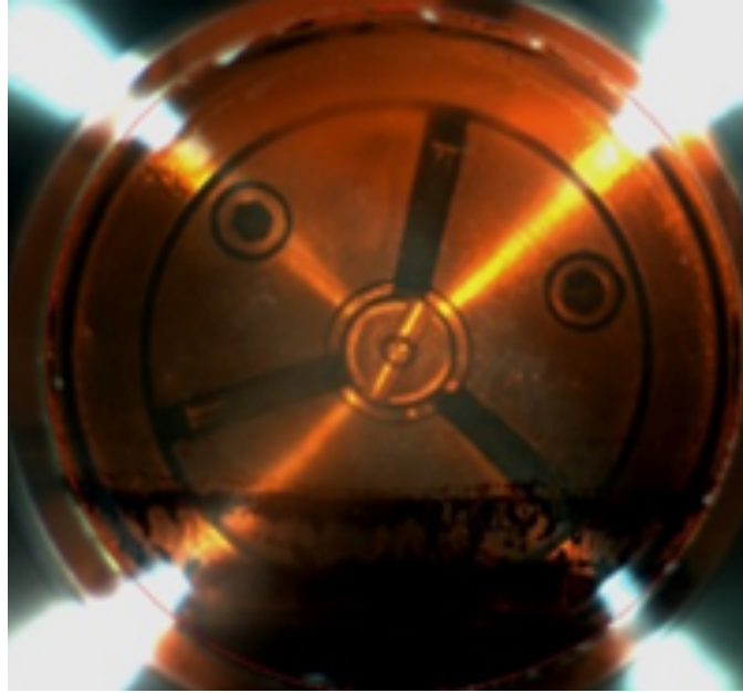
Figure 40 Miscible phase behavior at 4270.45 psi between CO 2 and oil at 120 °C
