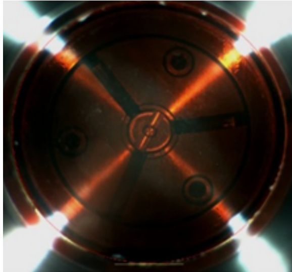
Figure 36 Miscible phase behavior at 4420.13 psi behaviors between CO 2 and oil at 80 °C
