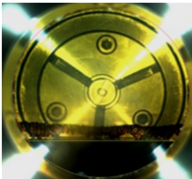
Figure 39 L 1 L 2 phase behavior at 3642.76 psi between CO 2 and oil at 120 °C
