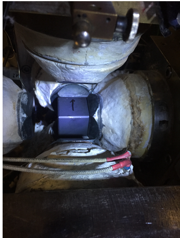
(b) True triaxial testing apparatus closeup view
