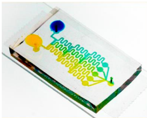
Figure 18. Simple cure PDMS microchannels full of different dye fluids representing a micro model, Reprinted with permission from 87 , ACS 2013
