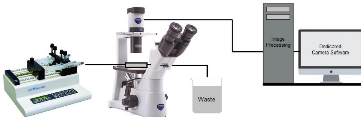
Figure 23. A basic microfluidic setup including microfluidic chip, inverted light microscope, camera, and image processing computer unit.
