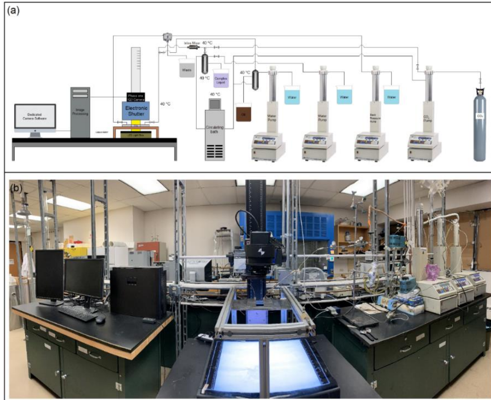
Figure 53. (a) schematic of high-pressure CO 2 foam injection and visualization of microchip in laboratorial scale; the system is capable of scCO 2 foam generation as well as oil injection through the microchips. The simultaneous visualization is performed by high resolution camera and fast processing units. (b) The photo of the actual setup in the lab in Professor Saman Aryana’s lab in Chemical Engineering Department, University of Wyoming, reprinted with permission from 121 JOVE 2020
