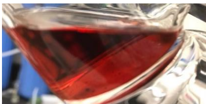
Figure 46. 1M Mn-3M H 2 SO 4 solution after the cyclic voltammetry experiment on graphite rod working electrode.
