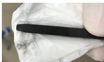
Figure 47. Graphite working electrode after the cyclic voltammetry of 1M Mn-3M \text{H}_2\text{SO}_4 solution
