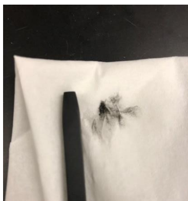
Figure 52. Graphite working electrode after the cyclic voltammetry of 1M Mn-3M H 2 SO 4 solution
