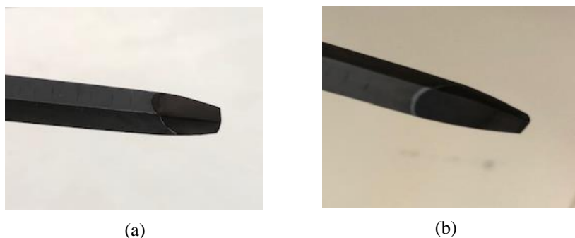
Figure 56. Pictures of the surface of the graphite rod working electrode after the anodic voltage hold experiment, (a) in 1M Mn-3M \text{H}_2\text{SO}_4 , (b) in 1M Mn-1M Ti-3M \text{H}_2\text{SO}_4
