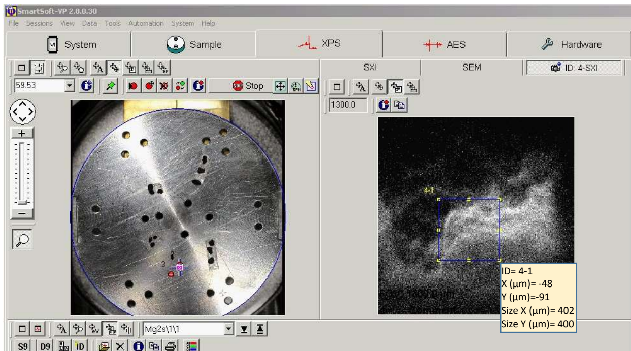
Figure 3-20: XPS standard sample studs (left) and specified area on sample surface to retrieve targeted atoms (right).
