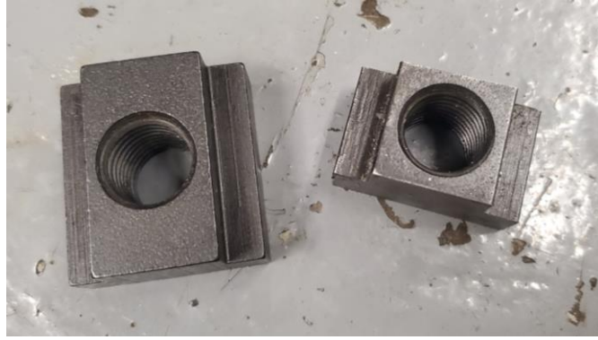
Figure 4.16: Original T-slot nut (left) and modified one (right)
