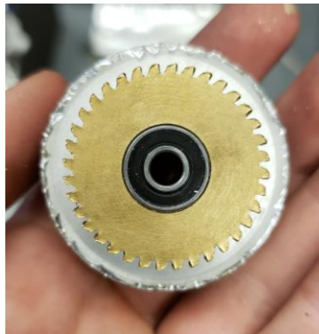
Figure 4.8: Damaged brass gear from vibration from engine test setup iteration #3
