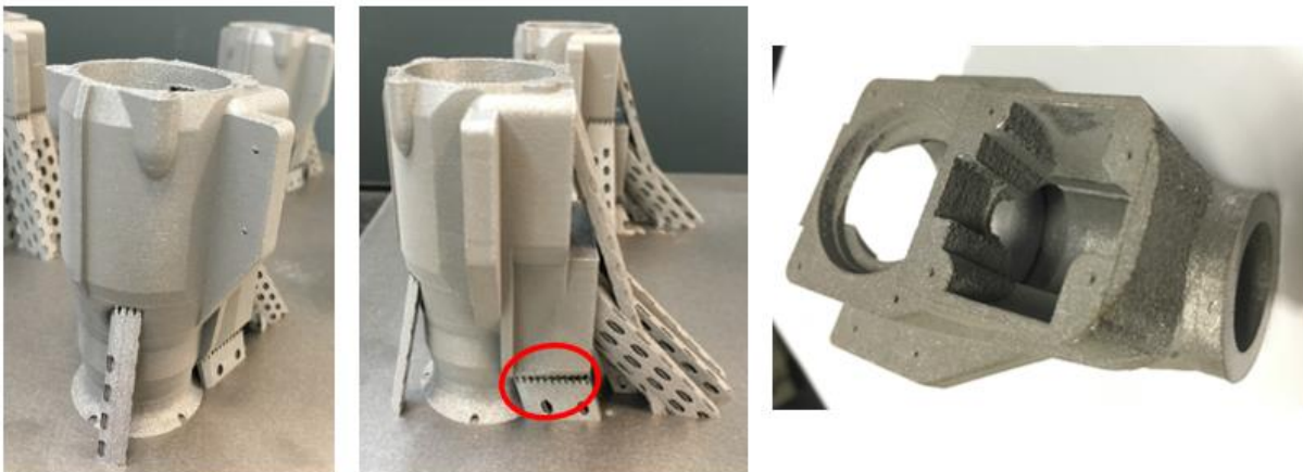
Figure 3.14: Modified crankcase build results
