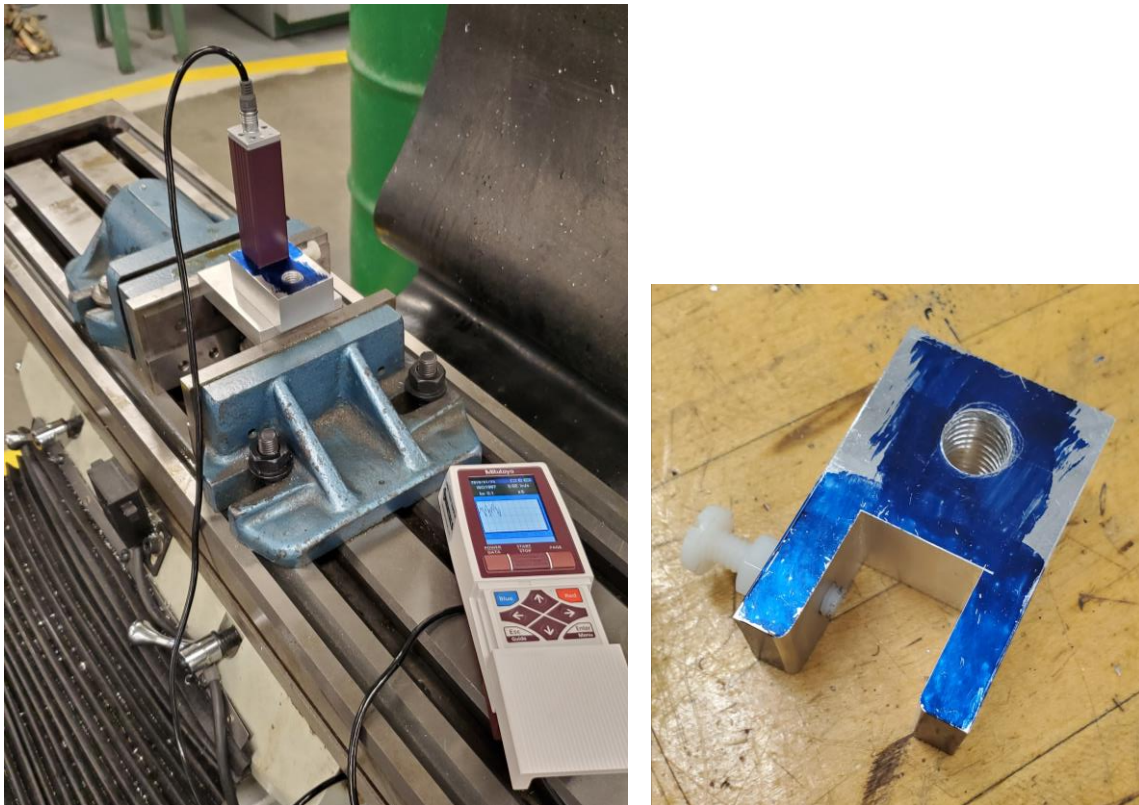
Figure 3.57: Profilometer measurement set up (left), and fixture for profilometer (right)
