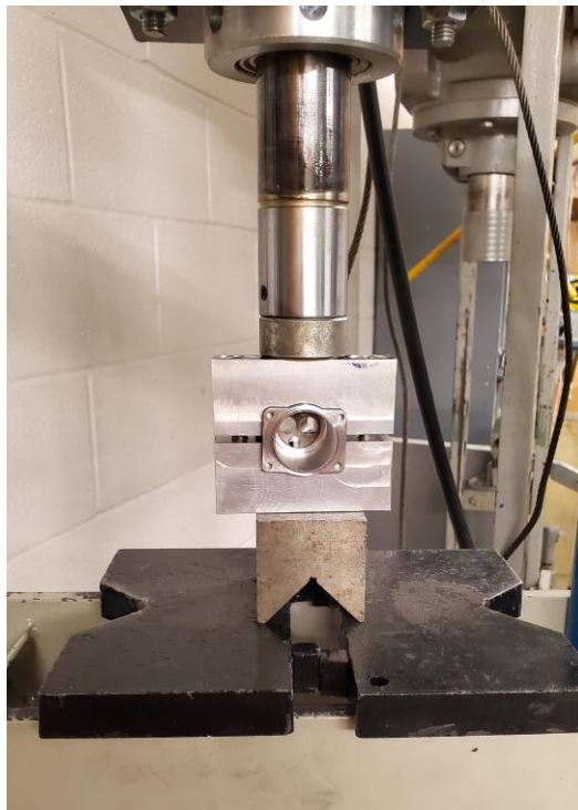
Figure 3.55: Using a hydraulic press to yield the cylinder back into a cylindrical shape
