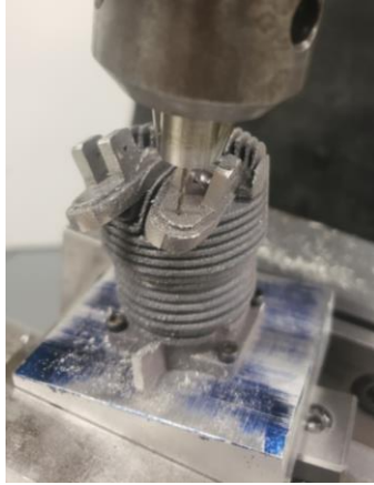
Figure 3.41: Set up for 10° angled features (feature 2) on cylinder head
