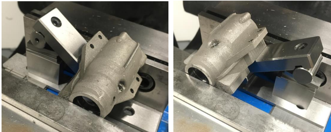
Figure 3.35: Vice placement using sine block for angled sensor holes (feature 20)
