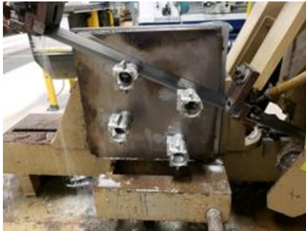
Figure 3.30: Build plate removal using a bandsaw
