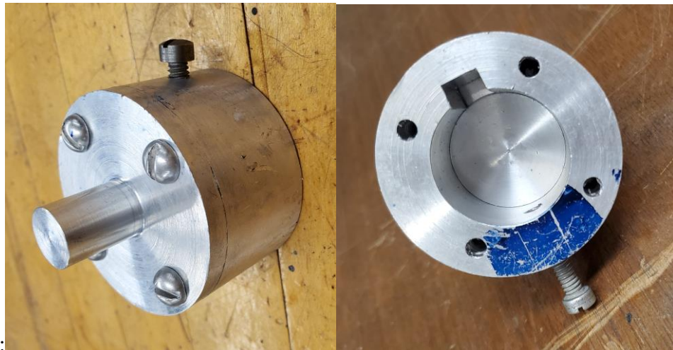
Figure 4.17: Futek sensor shaft reduction adaptor
