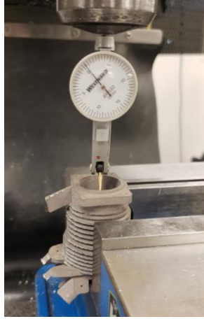
Figure 3.39: First vice set up to drill the initial four holes (feature 11) in the cylinder head
