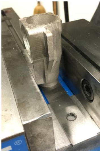
Figure 3.33: Vice placement for final squaring step and proceeding boring, reaming, drilling, and tapping steps (features 2, 3, and 11-14 machined with this set up)
