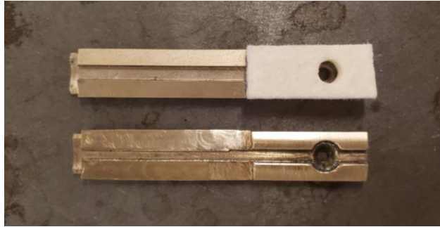
Figure 3.50: Modified bronze guide shoes for silicon exposure (top) and blind hole honing (top and bottom)
