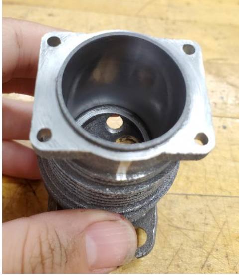
Figure 3.65: Finished (post honing process) AM cylinder wall
