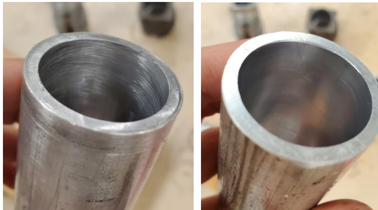
Figure 3.54: Practice honing: before bronze guide shoes were filed (left), and after (right)
