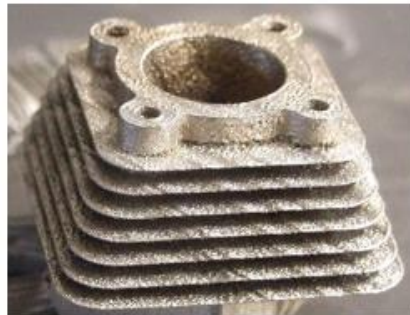
Figure 2.2: AM engine block produced with SLM technology [14]
