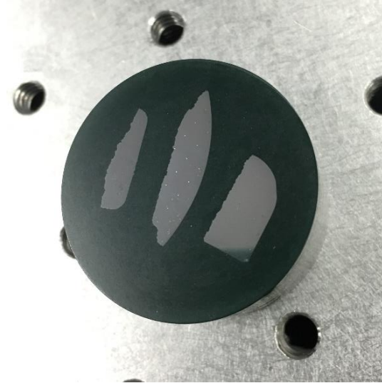
Figure B.1: Cylinder head broken fins used as a test specimen, polished to 1 \mu\text{m}
