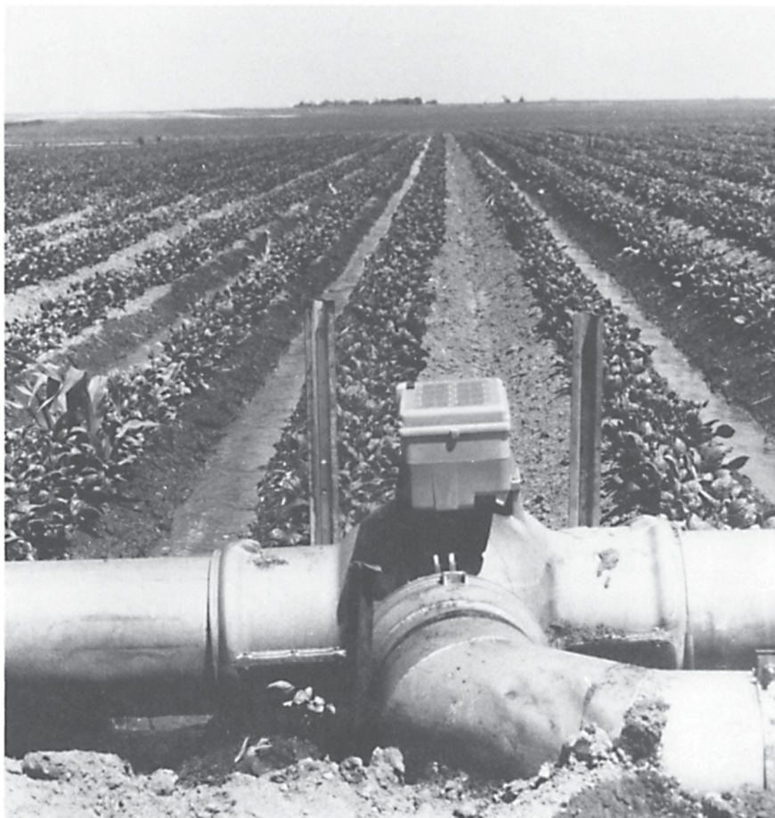
Surge-flow system with solar-powered controls on top. Chase County, Nebraska.
