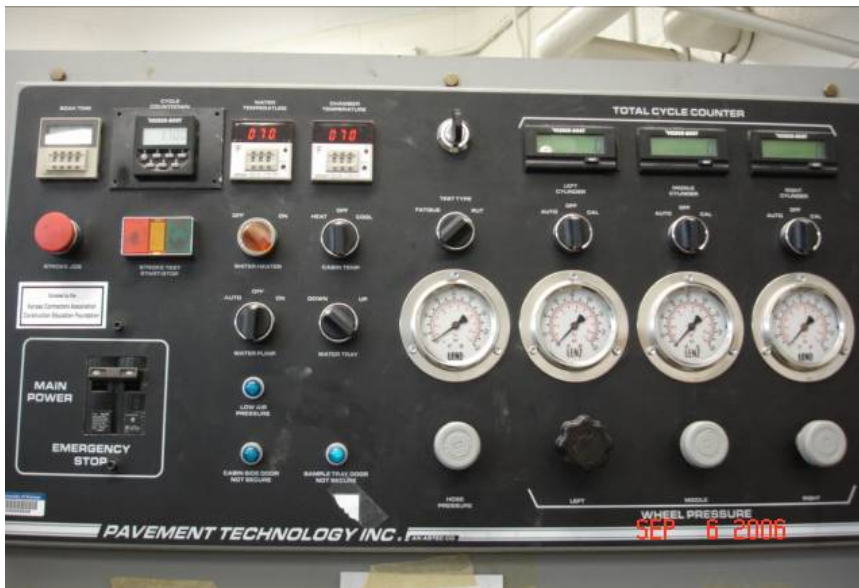
Figure 3-5 Control panel of APA
