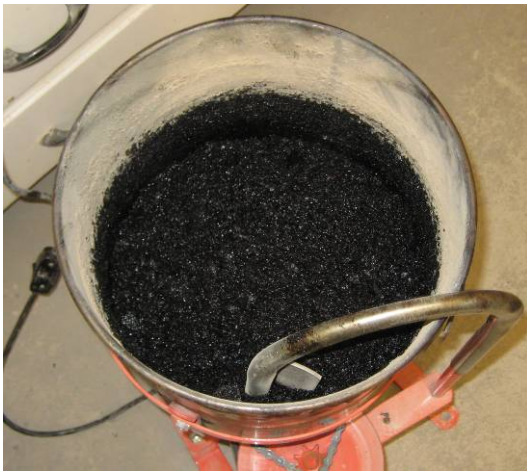
Figure 3-9 Mixing of aggregate and binder
