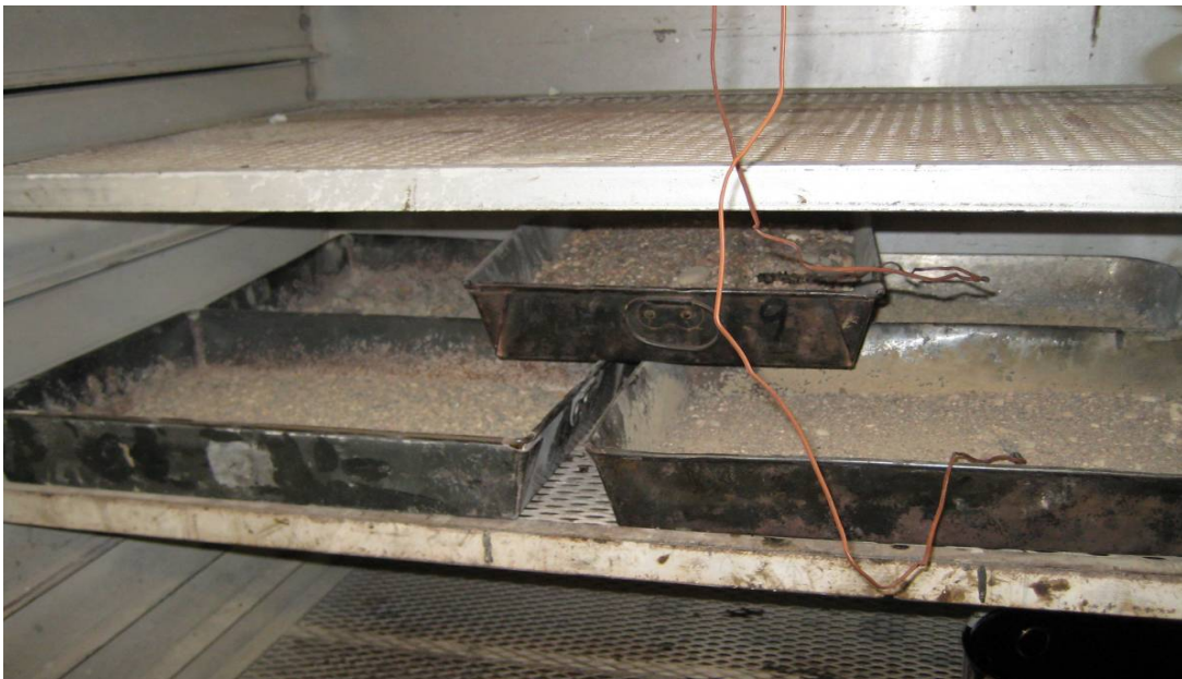
Figure 3-7 Heating of aggregate up to the required mixing temperature
