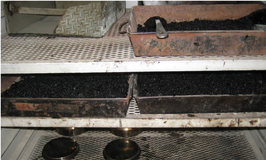
Figure 3-10 Short term aging of Superpave mix
