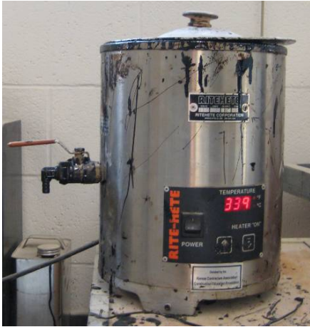
Figure 3-8 Heating of asphalt binder up to the required mixing temperature
