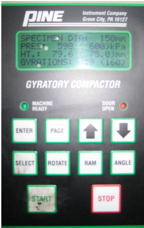
Figure 3-1 Pine Superpave Gyratory Compactor Control Panel
