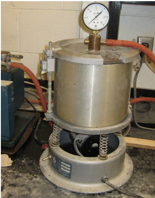
Figure 3-15 Vacuum saturation of a sample before wet testing
