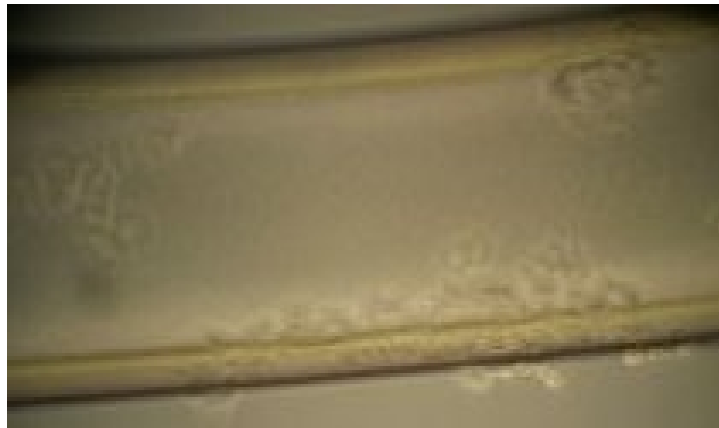
Figure 5.10. PAN membrane coated with the combination of fibronectin and poly-d-lysine. Probe was seeded with Bewo cells at a density of 150,000 cells/cm 2 on day one and day two. Probe was perfused with PBS at 2 \mu L/min.
