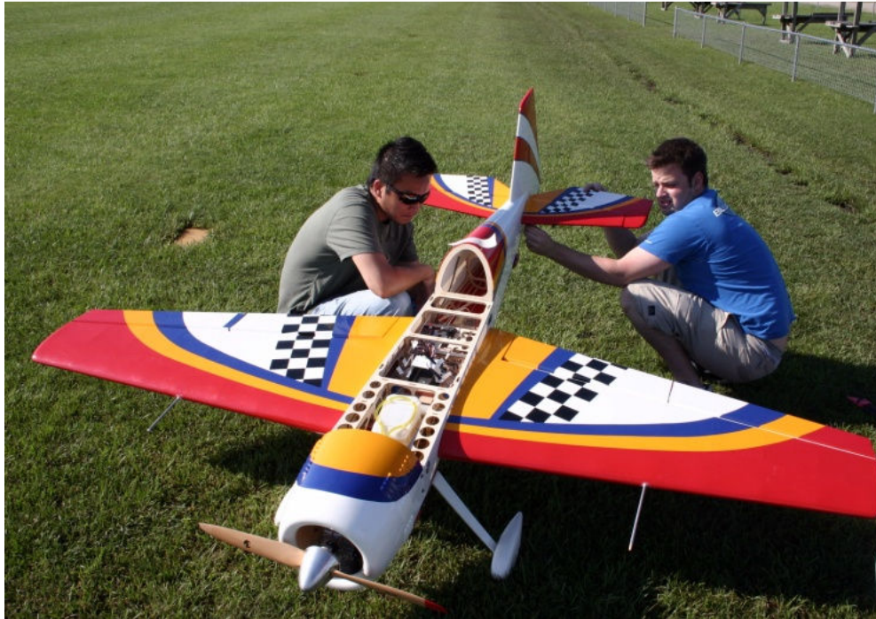
Figure 2-4: Yak-54 Model as a Test Platform for UAV Avionics
