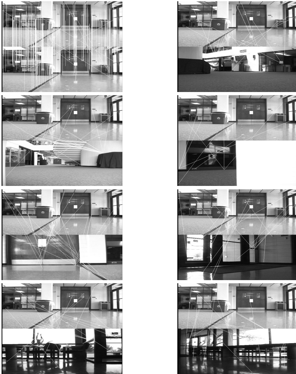
Figure 5.18: Geometric image matching. The sample images show how matches are made. The eight different images represent one image from each of the eight orientations (bottom) and the test image that was used to compare (top). Lines are drawn between matching keypoints. The number of lines represents the number of matches. The top left image, representing the image at zero degrees, matched the best in this case.
