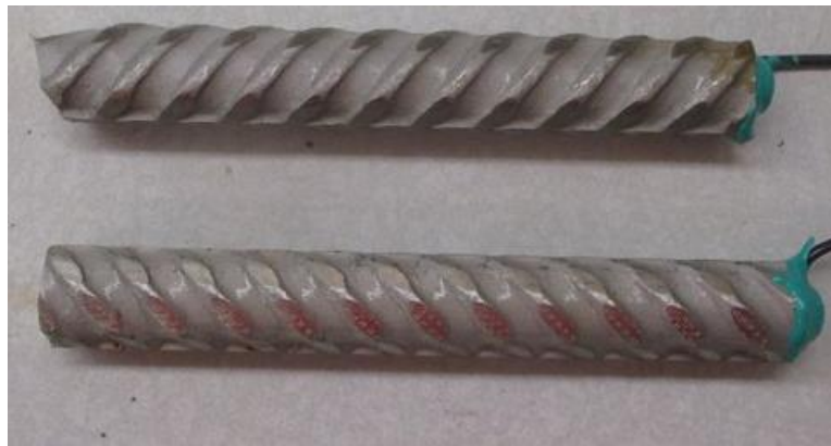
Figure 4: 2205 stainless steel reinforcement after one week of exposure to simulated seawater at 65 °F.
