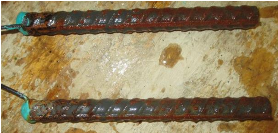
Figure 8: A1035-CM reinforcement after one week of exposure to simulated seawater at 50 °F.
