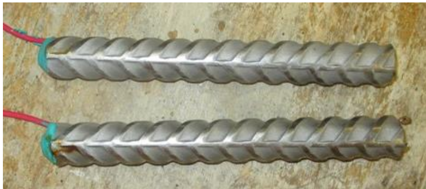
Figure 6: 2304 stainless steel reinforcement after one week of exposure to simulated seawater at 80 °F.
