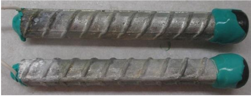
Figure 9: A1094 reinforcement after one week of exposure to simulated seawater at 65 °F.
