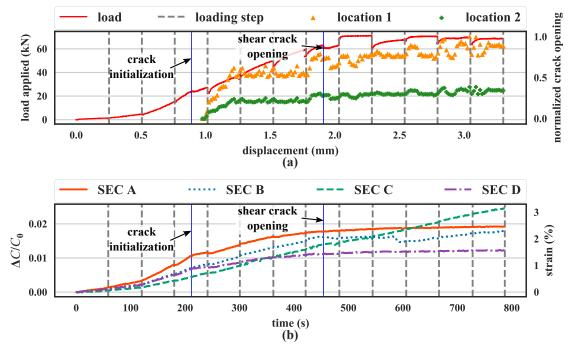
**Figure 4.** Time series results from the small-scale reinforced concrete beam: (a) load-displacement curve and normalized crack opening widths histories; and (b) relative capacitance and computed strain histories for all four SECs.
