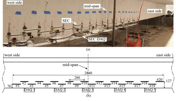
**Figure 8.** Sensor instrumentation around the midspan of the beam: (a) picture; and (b) schematic of sensor locations, partial beam elevation (dimensions are in mm).
