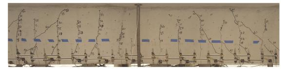
Figure 9. Picture of crack pattern before reaching ultimate strength after loading step 19.
