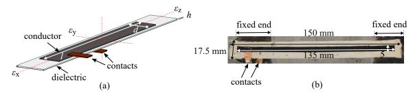
**Figure 1.** (a) Schematic representation of an SEC; (b) picture of an SEC with active sensing area measuring  $135 \text{ mm} \times 5 \text{ mm}$ .
