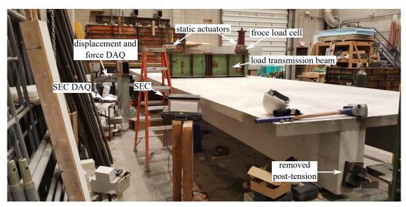
Figure 6. Picture showing the experimental setup of the large-scale post-tension beam test setup.
