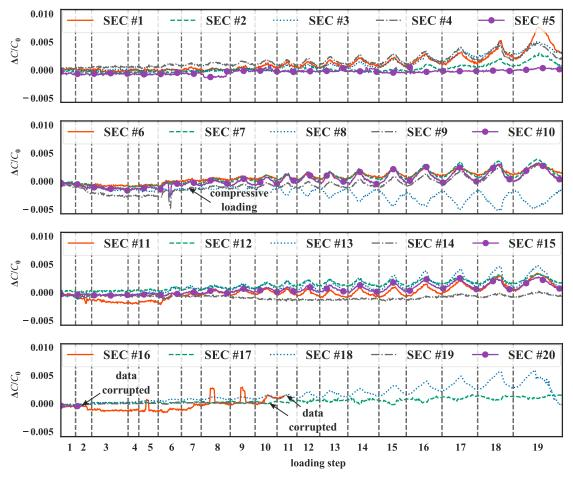
Figure 10. Time histories of strain measurements for all SECs.
