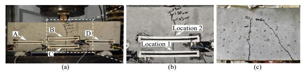
**Figure 3.** (a) Crack patterns on the small-scale reinforced concrete beam; (b) an enlarged view of the cracks on the front side of the specimen; and (c) an enlarged view of the cracks on the back side of the specimen showing a shear crack.
