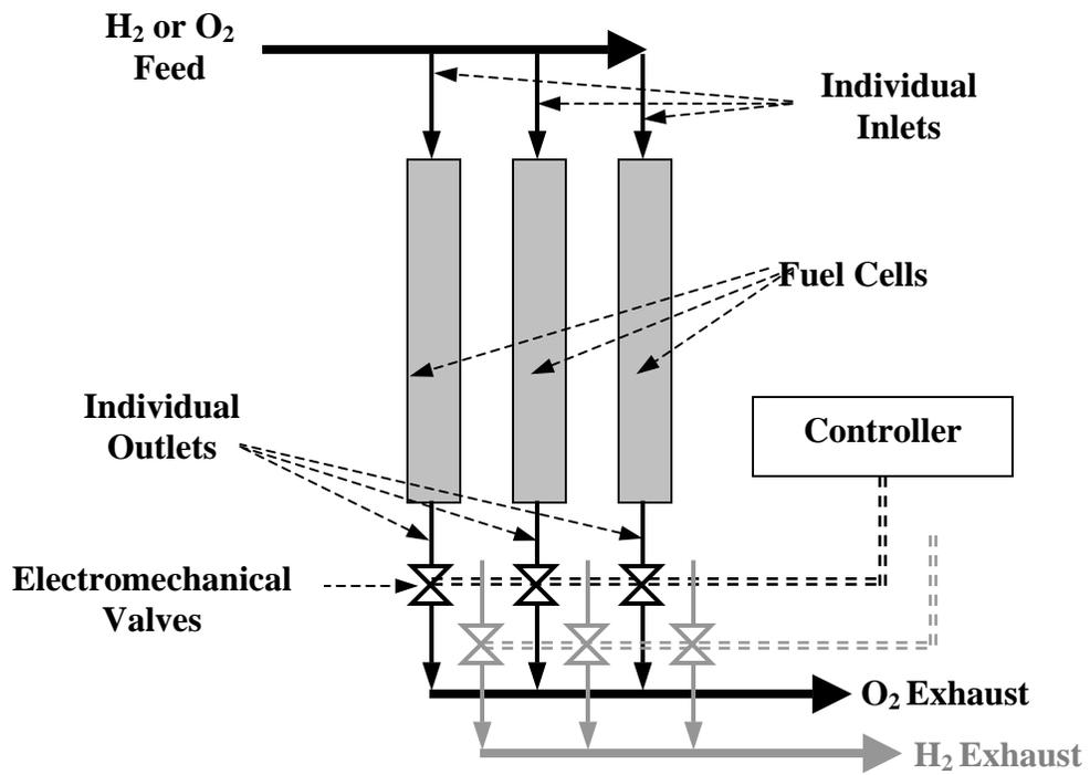
*Figure 4. Fuel Cell Stack with Sequential Exhaust System Using Electromechanical Devices.*
