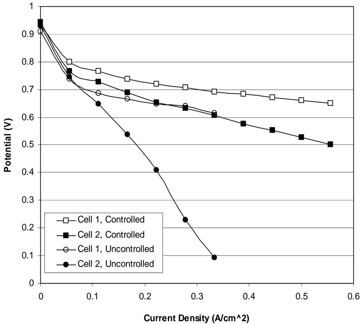
**Figure 6.** Polarization Curve Comparison of a Two-Cell Stack Operating With and Without Sequential Exhaust Control. Cell temperature  $\approx 35^{\circ}$ - $40^{\circ}$ C,  $H_2$  flow rate =  $1.5A/cm^2$  equivalent,  $O_2$  flow rate =  $2.0 A/cm^2$  equivalent.
