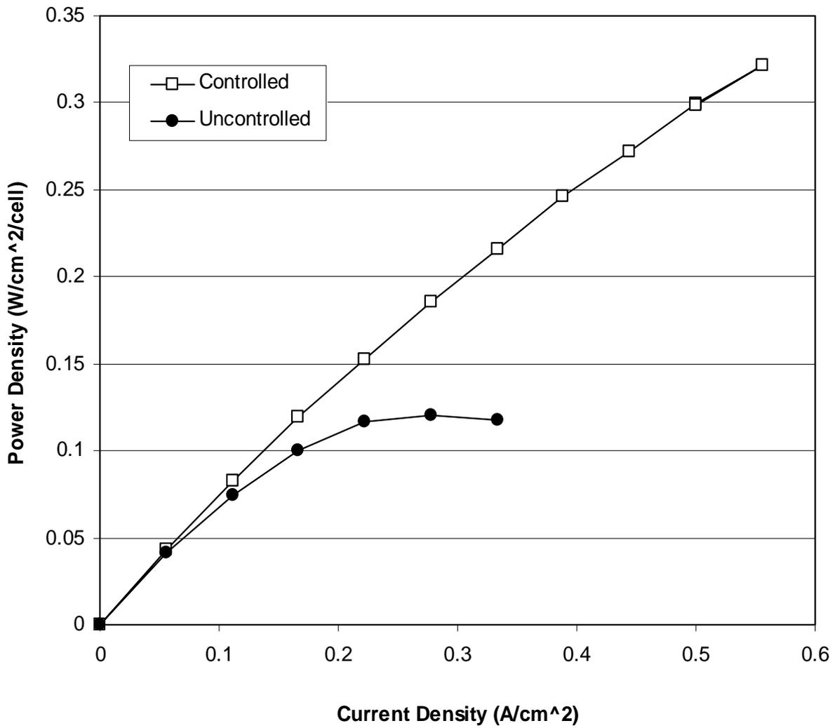
**Figure 5.** Power Density Comparison of a Two-Cell Stack Operating With and Without Sequential Exhaust Control. Cell temperature  $\approx 35^{\circ}$ - $40^{\circ}$  C,  $H_2$  flow rate =  $1.5 A/cm^2$  equivalent,  $O_2$  flow rate =  $2.0 A/cm^2$  equivalent.
