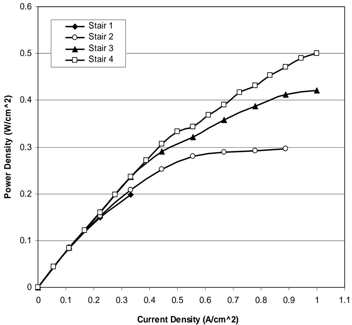
**Figure 7.** Recovery of a Two-Cell Stack from Flooded Conditions by Using a Sequential Exhausting Device. Cell temperature  $\approx 35^{\circ}$ - $40^{\circ}$ C,  $H_2$  flow rate =  $1.5A/cm^2$  equivalent,  $O_2$  flow rate =  $2.0 A/cm^2$  equivalent.
