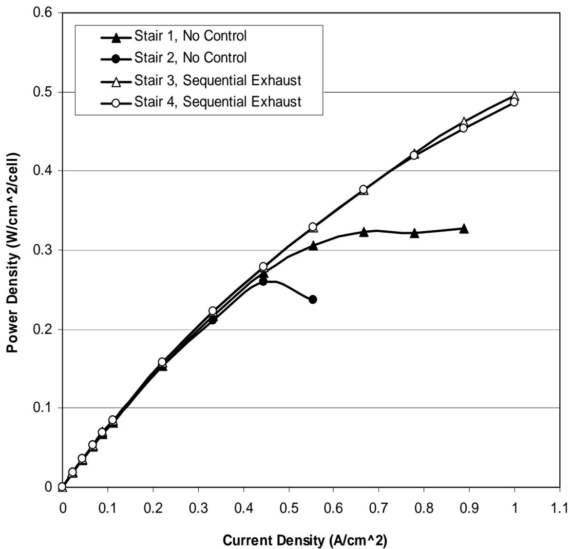
**Figure 8.** Power Density Comparison of a Three-Cell Stack Operating With and Without Sequential Exhaust Control. Cell temperature  $\approx 35^{\circ}$ - $40^{\circ}$ C, for  $H_2$  and  $O_2$  flow rates see Table I.
