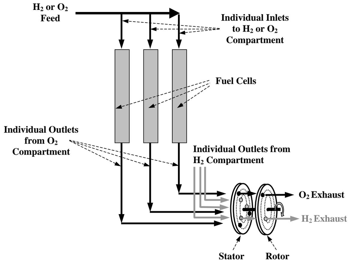
*Figure 3. Fuel Cell Stack with Sequential Exhaust System Employing a Rotating Device.*
