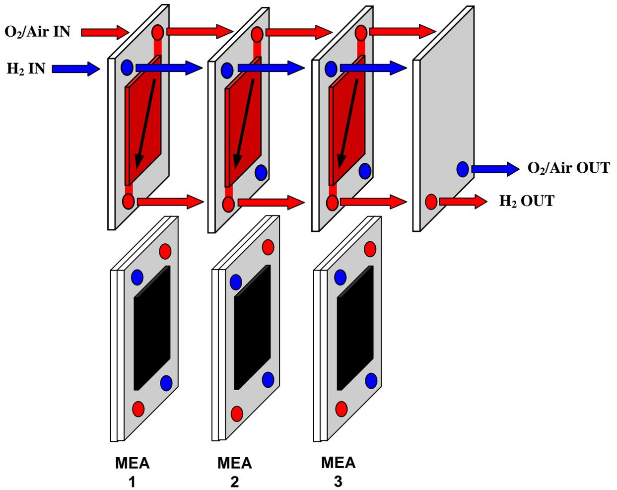
*Figure 2. Fuel Cell Stack with Parallel Gas Feed and Exhaust.*
