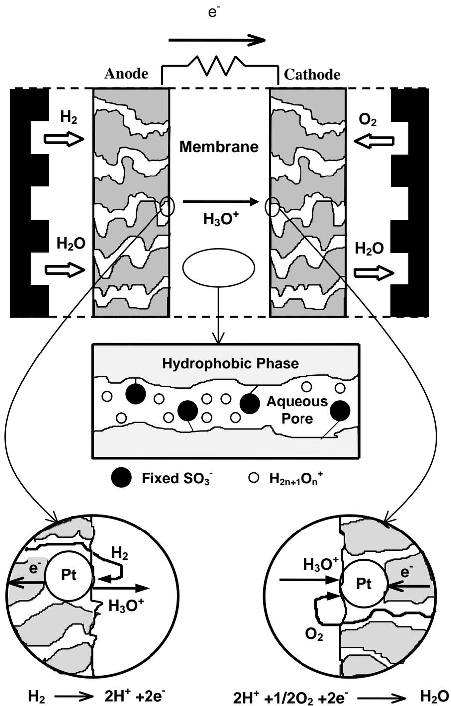
Figure 1. Processes of Polymer Electrolyte Fuel Cell
