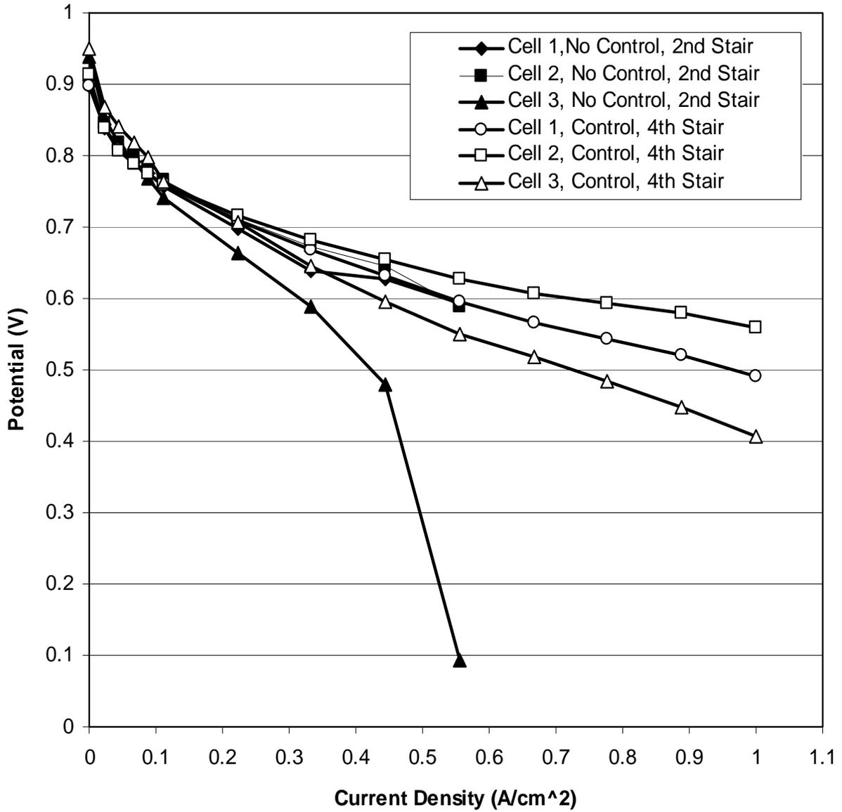
**Figure 9.** Polarization Curve Comparison of a Three-Cell Stack Operating With and Without Sequential Exhaust Control. Cell temperature  $\approx 35^{\circ}$ - $40^{\circ}$ C, for  $H_2$  and  $O_2$  flow rates see Table I.
