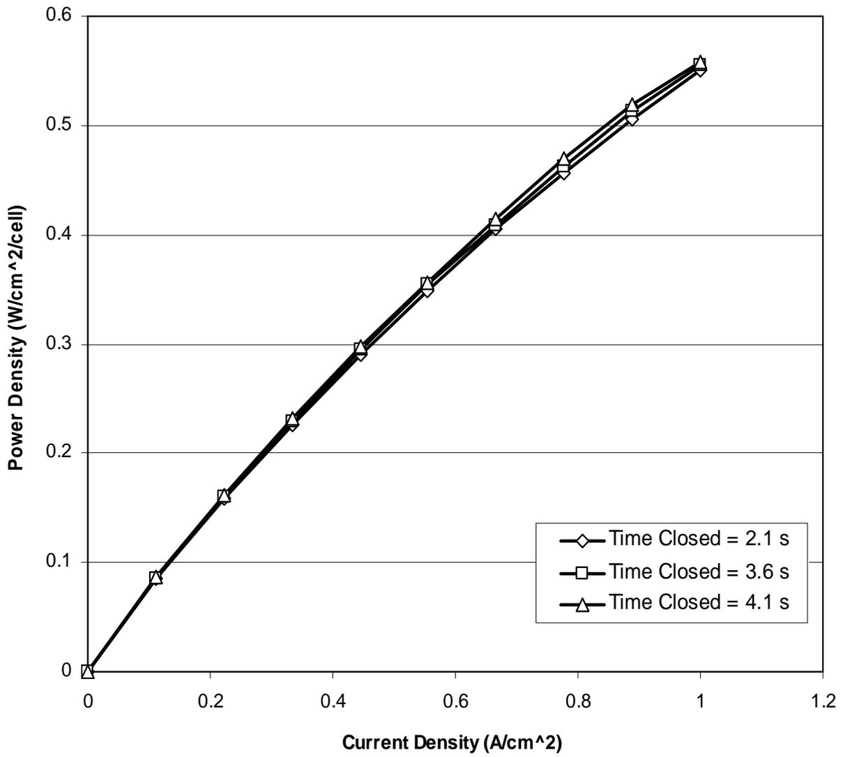
**Figure 10.** The Effect of Varied Valve Closed Time Intervals on the Performance of a Three-Cell Stack. Time Open = 0.3 s.
