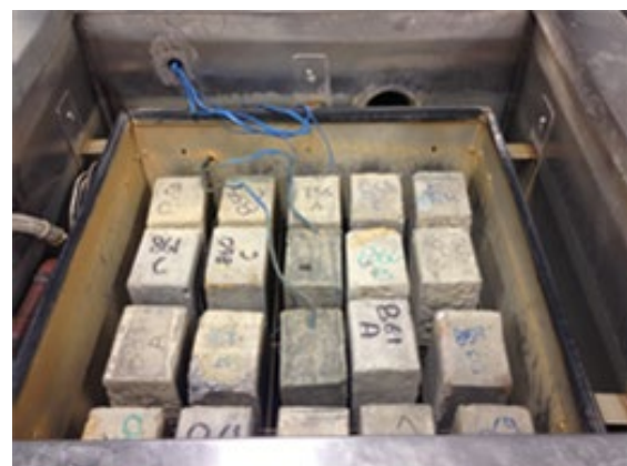
Figure 2.7 – Freeze-Thaw machine (Pendergrass and Darwin 2014)
