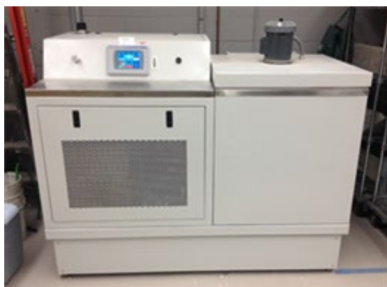
Figure 2.7 – Freeze-Thaw machine (Pendergrass and Darwin 2014)
