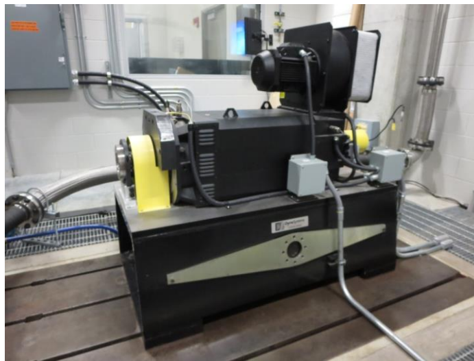
Figure C2. Dyne Systems 351 hp 3-phase AC dynamometer.
