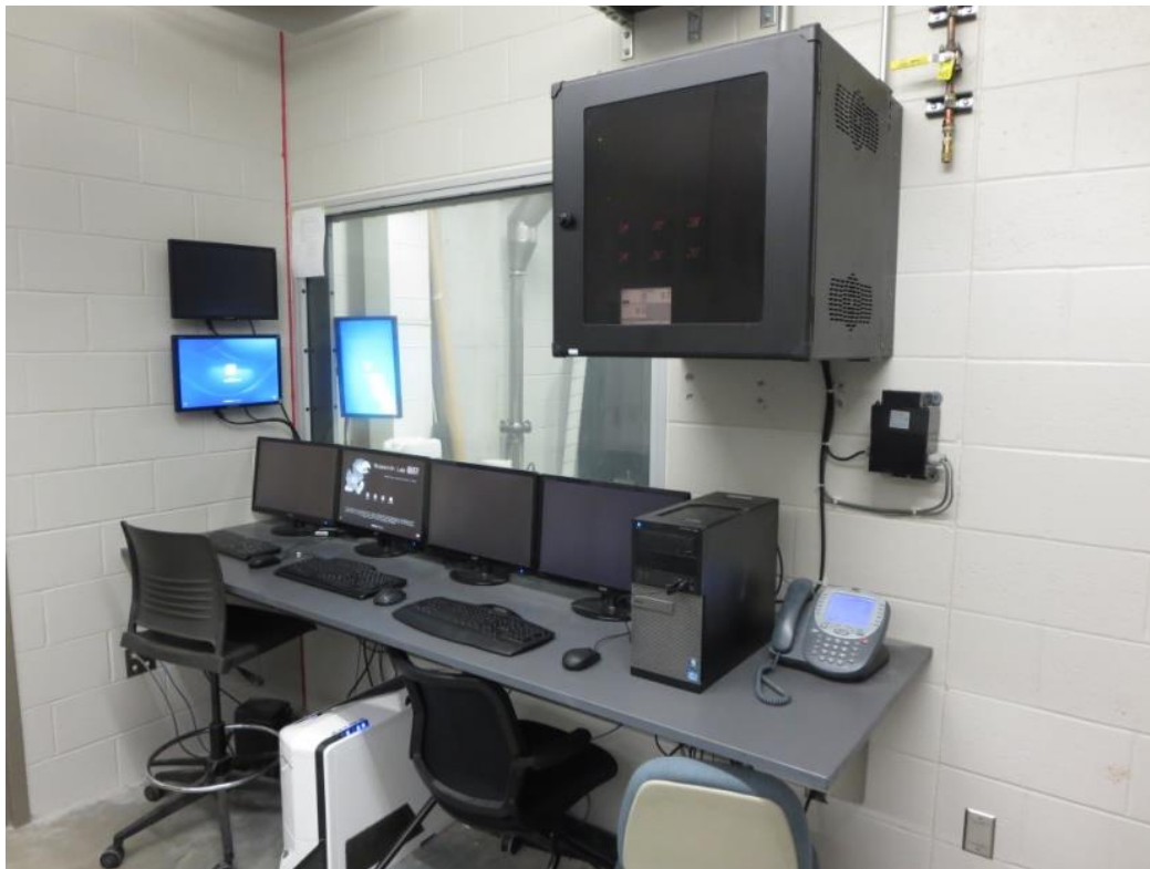
Figure C12. Multi-cylinder control room, adjacent the test cell.
