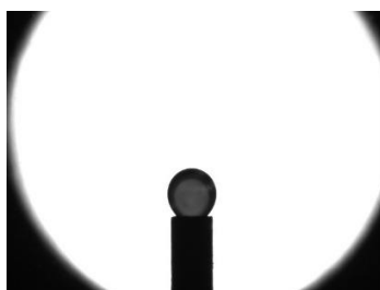
Figure 18 Hanging drop of MLP crude oil in 1% PEI pH=8
