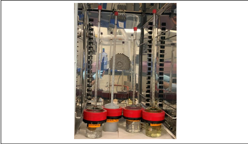
Figure 10 Amott test cells setup in oven at 40 degree Celsius
