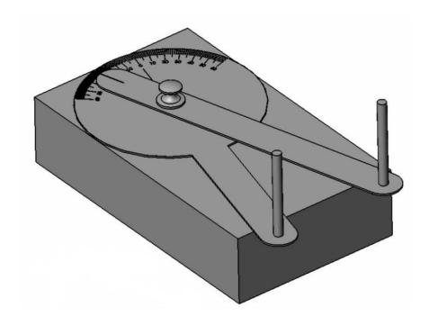
**Figure 2.1.** Schematic representation of the pinch aperture proprioception device.
