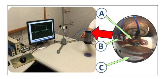
**Figure 4.1.** Experimental setting and the instrumented object. (A) uniaxial force sensor to register grip forces; (B) three-axial accelerometer to measure kinematic and gravitational accelerations in three dimensions (X, Y, and Z axes; (C) grasping surface (plastic pads).
