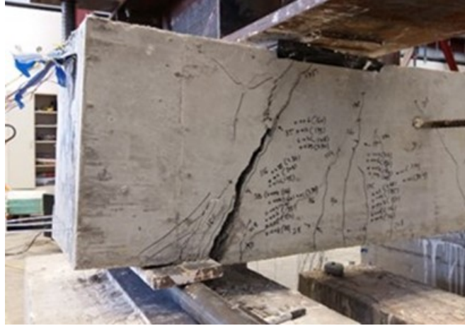
Figure 3.7 Pullout failure – Specimen H-3-8-5-11-F4.1-2
