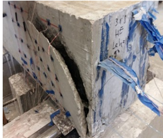
Figure 3.5 Side-face blowout failure – Specimen H-3-8-5-13-F4.1-2
