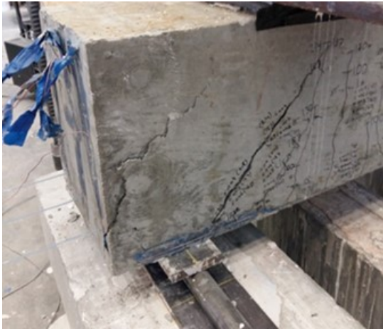
Figure 3.5 Side-face blowout failure – Specimen H-3-8-5-13-F4.1-2
