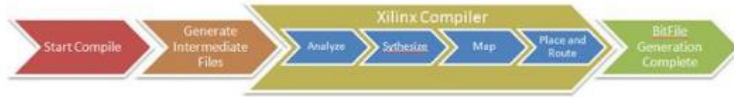
Figure 5.15: FPGA Hardware compilation steps [45].
