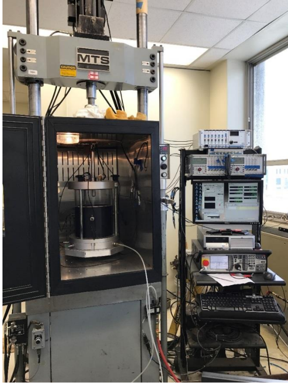
Figure 2-10: Material Testing System (MTS) with a triaxial cell and environmental chamber
