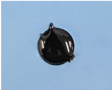
Figure 2-6: Binder sample for lower than 40 °C FS tests.
