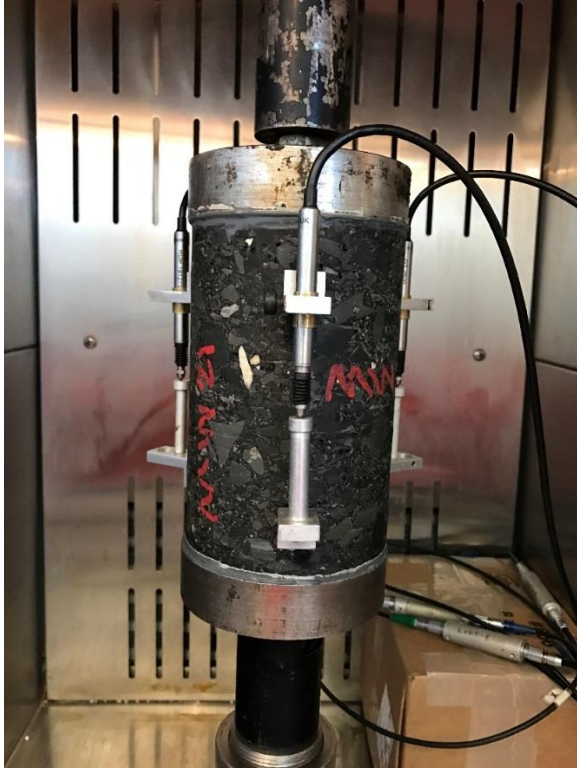
Figure 2-17: Experimental test setup for UCSR-T.
