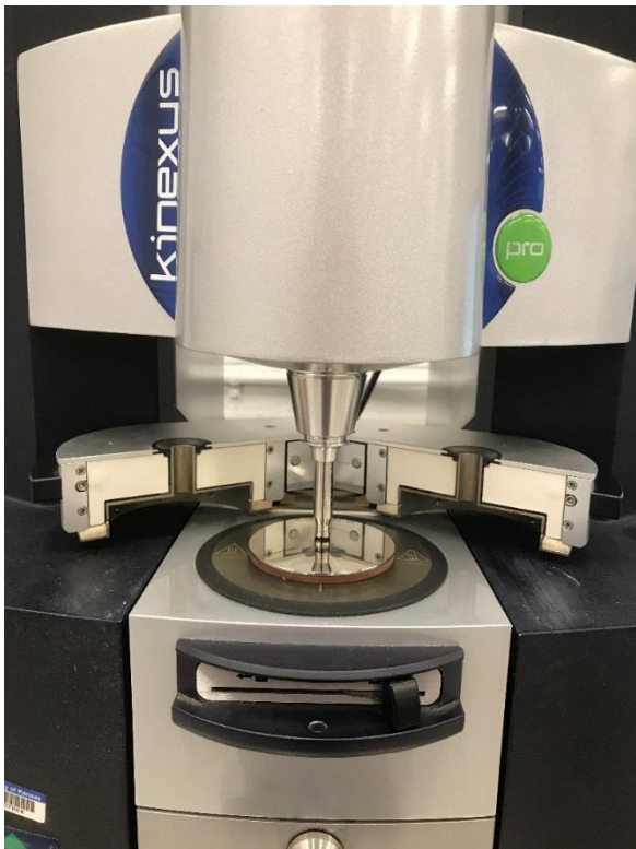
Figure 2-7: Binder sample for lower than 40 °C before FS tests using DSR
