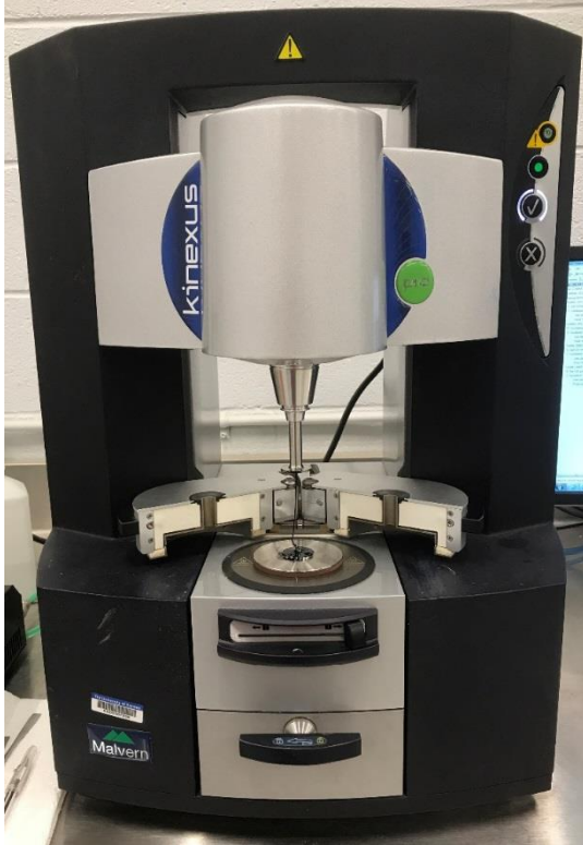
Figure 2-5: Binder sample after MSCR tests using DSR
