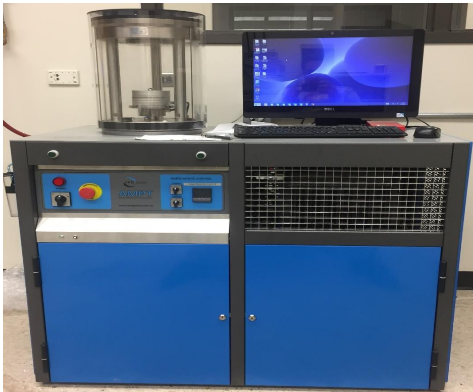
Figure 2-8: Asphalt mixture performance tester (AMPT)
