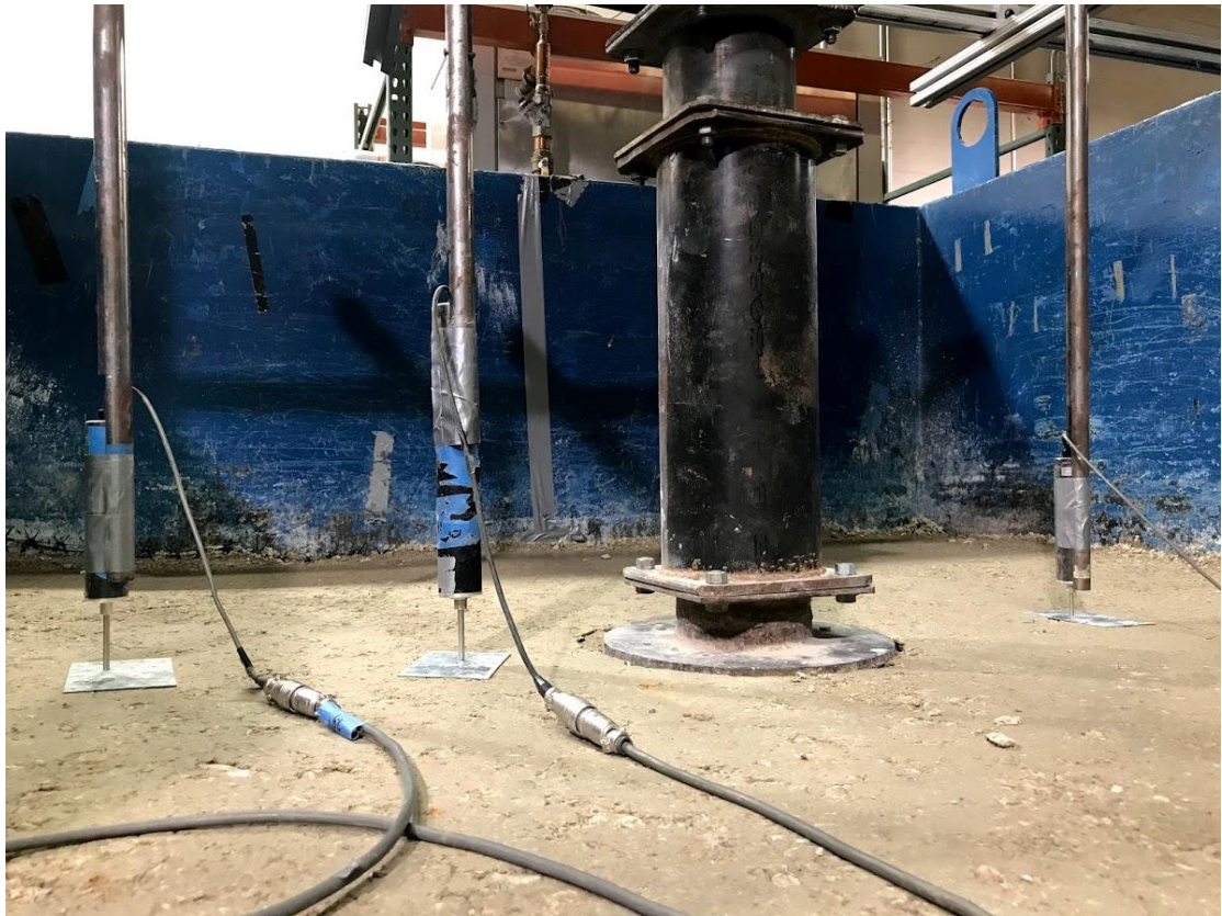
Figure 4.4 VGB test section showing punching of the loading plate
