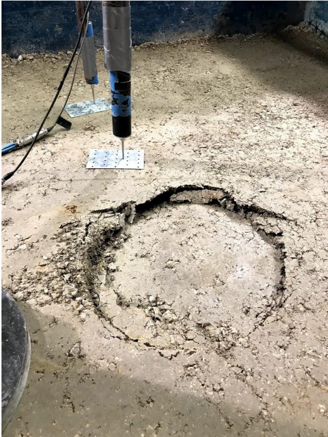
Figure 4.5 Top view of the VGB test section punched by the loading plate
