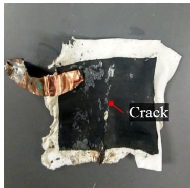
Figure 41. (a) SEC a1 was removed after 79,200 load cycles for a detailed inspection. On the bonded side (the side in direct contact with the steel surface) of the SEC, a crack was identified in the conductive layer, indicating damage to the SEC. The white color along the crack is the exposed dielectric layer.
