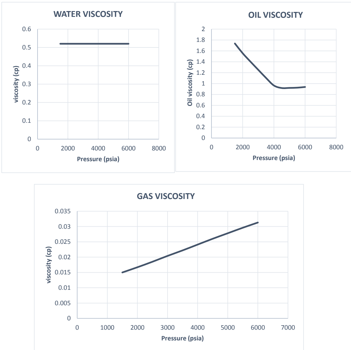
Figure 10. Fluid viscosities for A-1 formation
