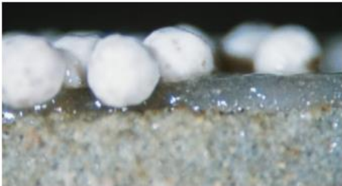
Figure 29. Filter cake build up after flowing 35 ppt CMHPG Zr XL fluid with breaker (StimLab Consortium Notes [49])
