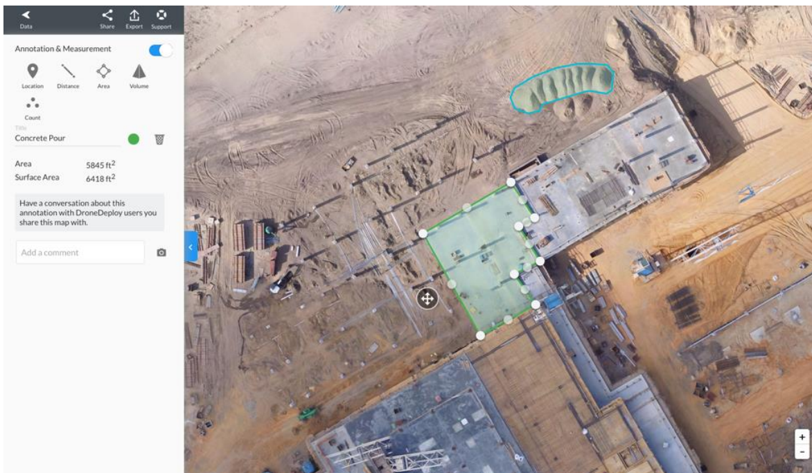
FIGURE 5.3. Drone-deploy software snapshot showing volumetric data analysis options.
